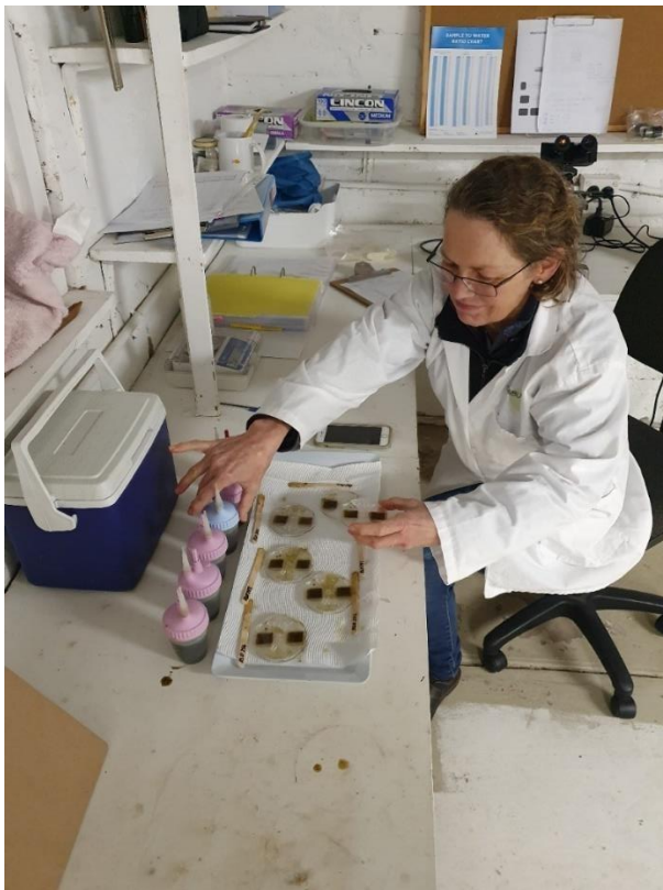
Figure 3: Investigator Sandra Playford preparing Mini-FLOTAC slides for worm egg counts using microscope at the Razorback Laboratory. Note use of Fill-FLOTAC for sample homogenisation and slide filling.
