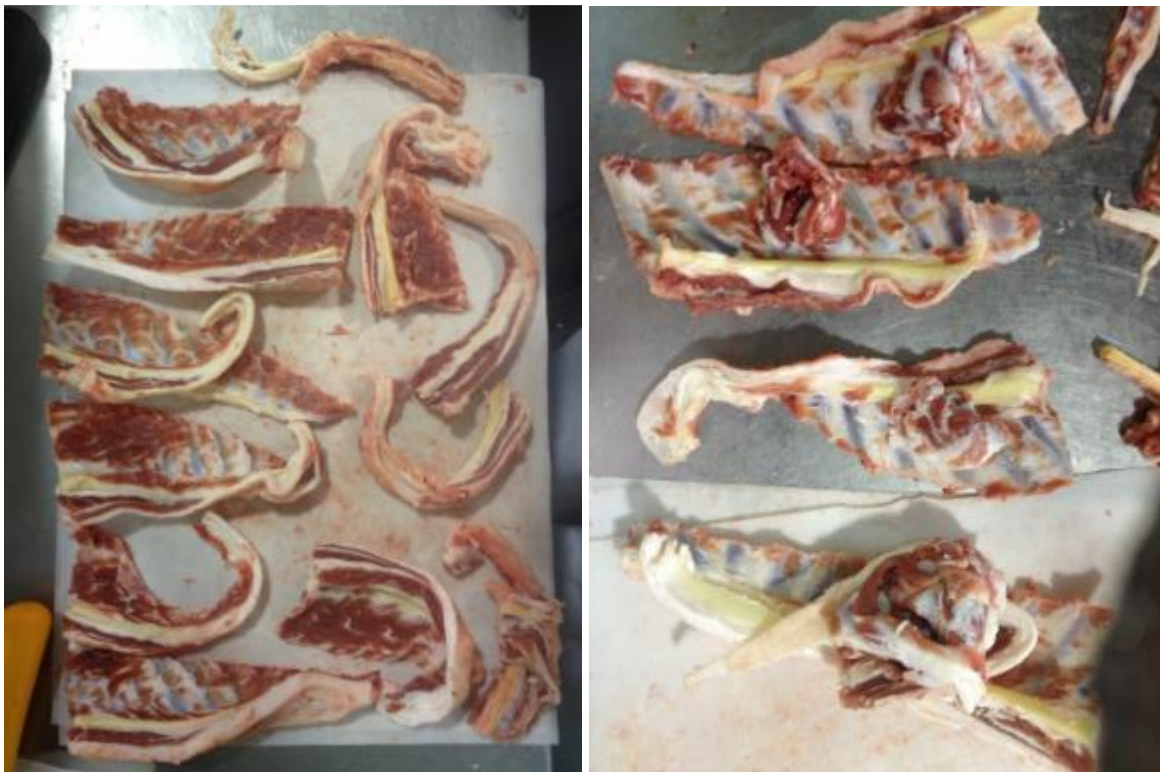
Figure 36: Chine bones from manual bandsaw process directly after chining, prior to scraping bones (left) and after scraping (right)
