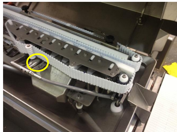
Figure 3: Water frenching jet (circled in yellow)
