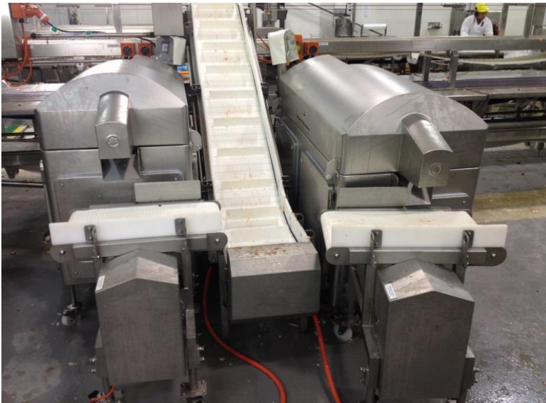
Figure 15: Foot print required by the two iFrenching system installed
