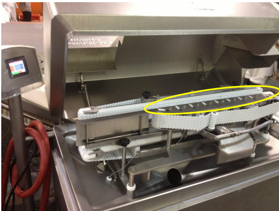
Figure 10: Mechanisms in the iFrenching system to modify the frenching length, shown by the yellow circles
