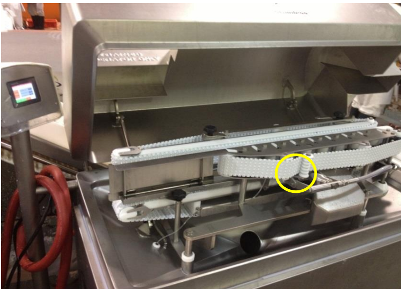
Figure 14: Lamb iFrenching water jets, shown by the yellow circle.
