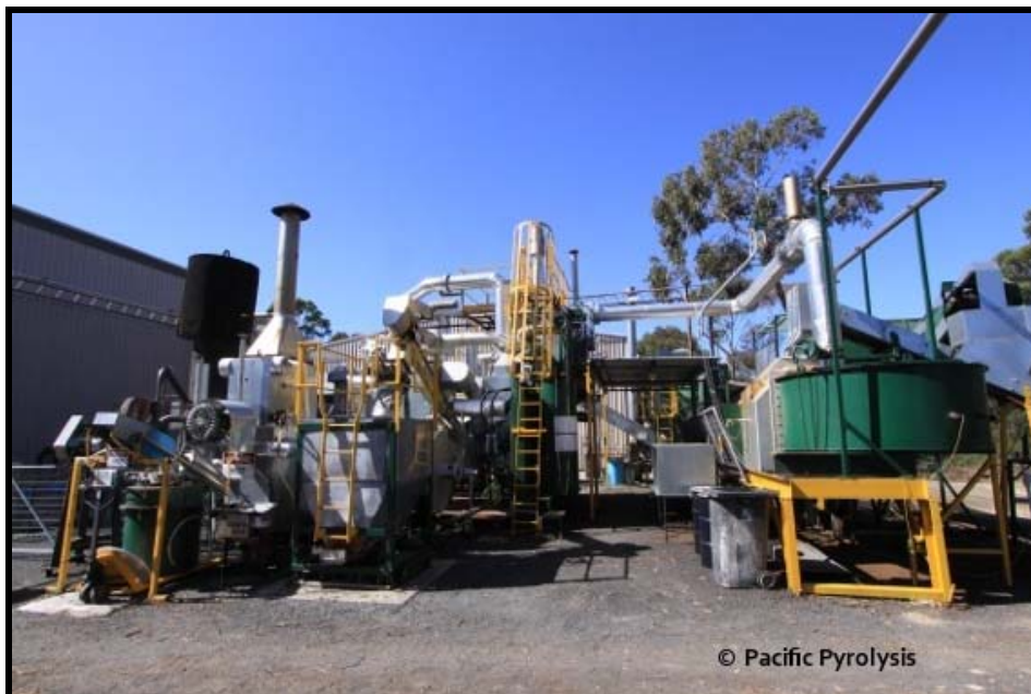
Figure 4.22: PacPyro 300 kg/h Pyrolysis Pilot Plant
