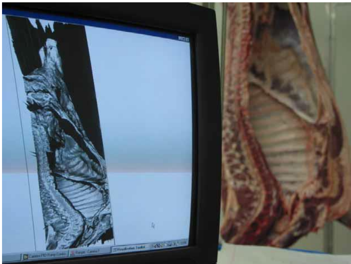
Figure 2-1 – Laser Surface Profile Scan, Carcass in Background (Unpublished photo, 2004, copyright Food Science Australia)
