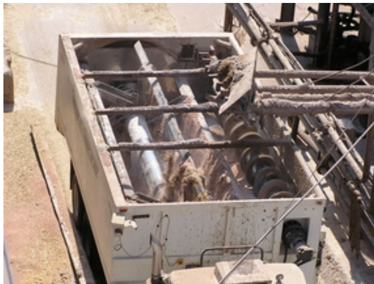
Photograph 11 - Truck mounted 920 -18 'Roto-mix' mixer feeder
