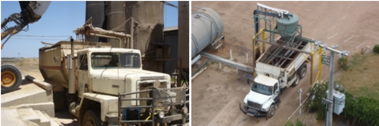
Photograph 14 - The liquid commodities may be individually Loaded (left) or Batched (right)
