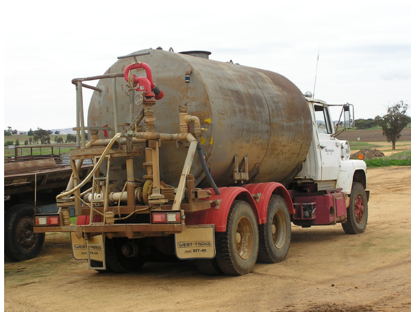
Photograph 20 - Water truck for road maintenance and dust suppression
