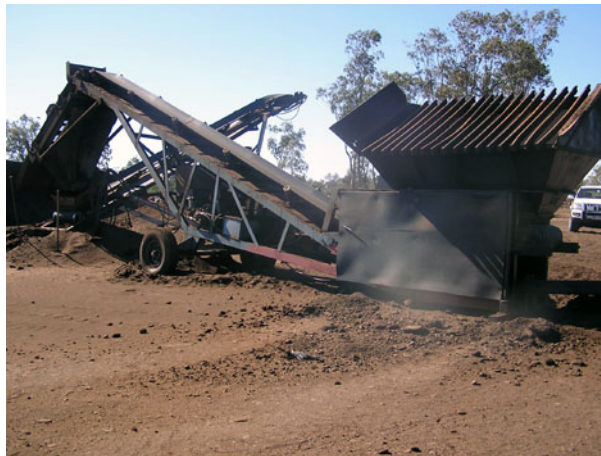
Photograph 18 – Screening machinery at manure stockpile
