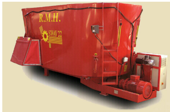
Photograph 6 - RMH stationary horizontal mixer suited for smaller feedlots (RMH, 2003).
