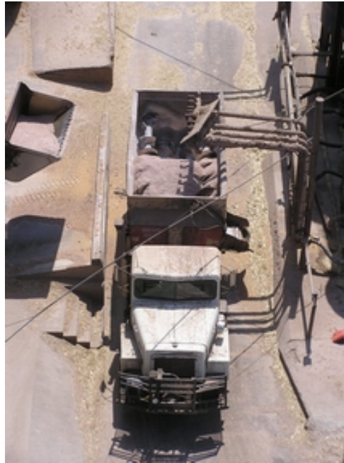
Photograph 9 - Truck mounted with a RMH David Evans Group screw feed mixer.
