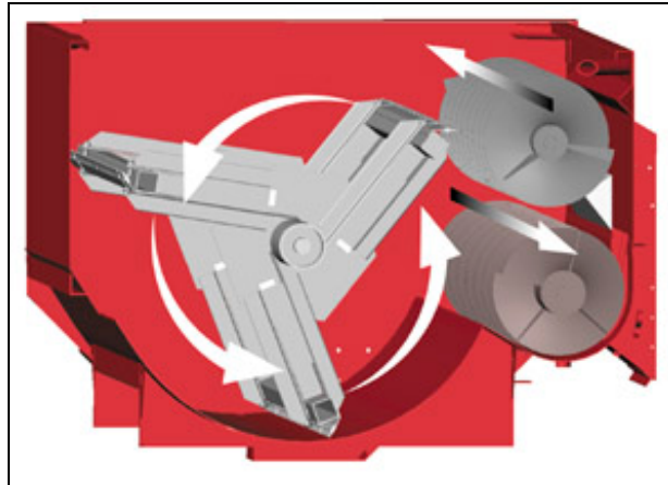
Photograph 10 - Diagrammatic representation of the Paddle Type ROTO-mix (ROTO-MIX, 2006).
