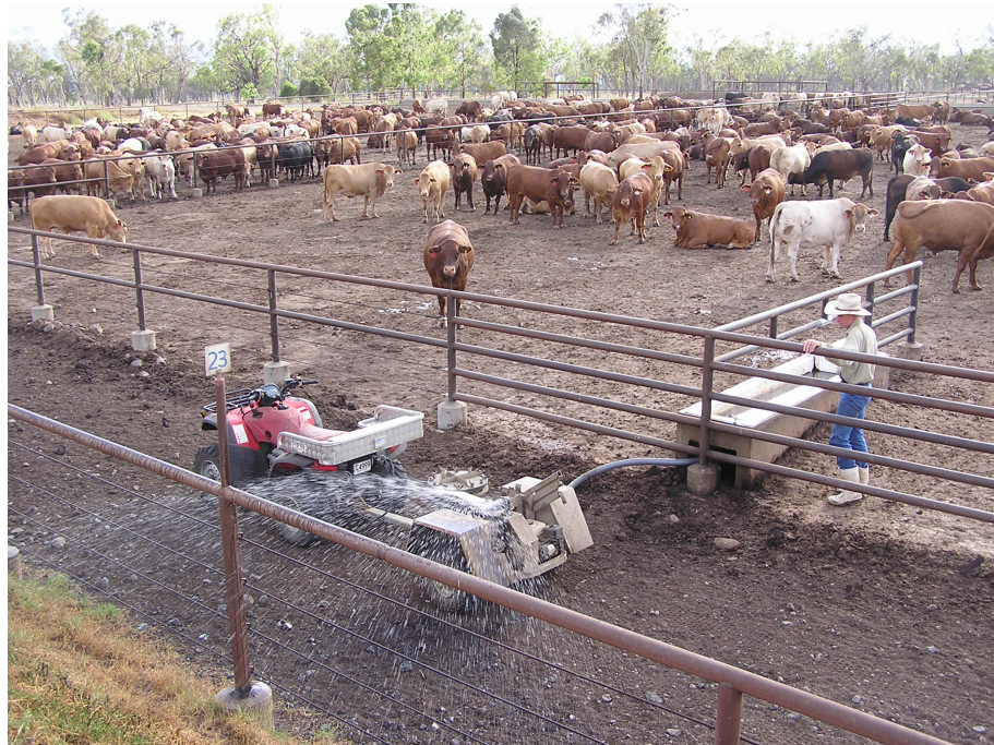
Photograph 64 – Trough cleaning process showing trailer mounted pump (Feedlot G)
