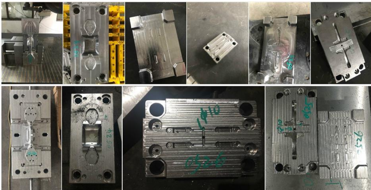
The ring only applicator mould tools in manufacture
