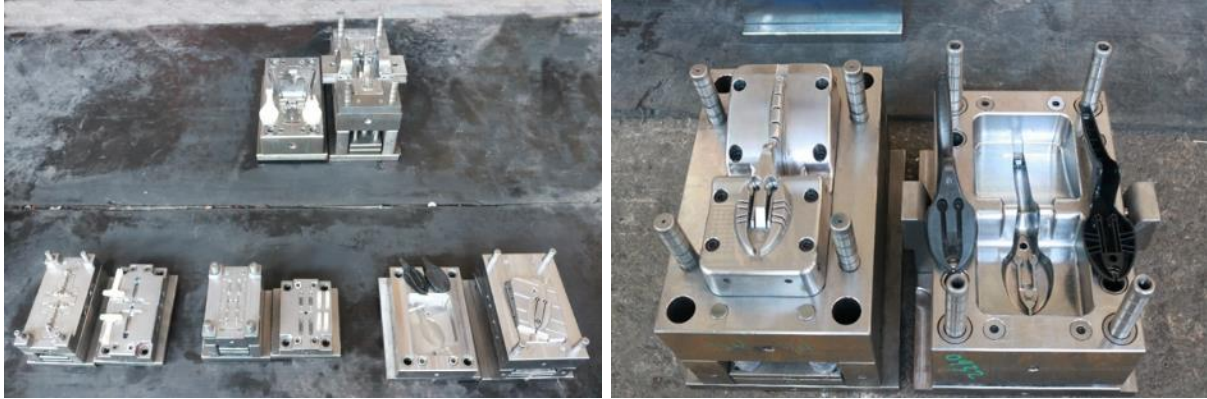
The mould tools for the ring only applicator
