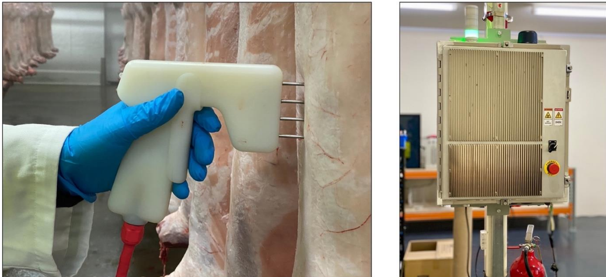
Figure 1. (left) Handpiece, comprising 4 needles to perform multiple measurements simultaneously. (right) Console that is connected to the handpiece, mounted on a stainless-steel pole.
