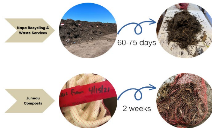
Figure 2: Cruz Foam before and after industrial composting. Top: Napa Recycling & Waste Services, Bottom: Juneau Composts
