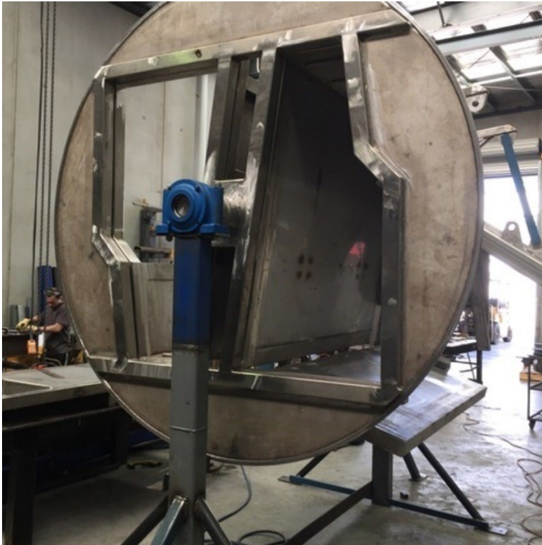
Figure 4: View of animal access to rotating restraint box, from rear. Image taken during workshop construction. In this image, the upright side is to the left, and the inverted side to the right.
