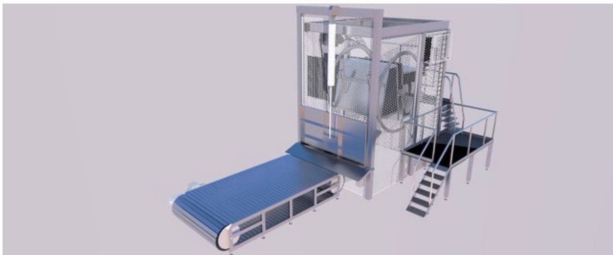
Figure 8: 3D representation of the rotating restraint box within the Faraday cage. Personnel access steps are on the right side of the image, with the bleed conveyor to the left.
