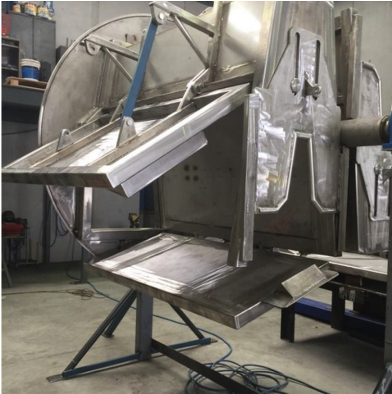
Figure 7: View of the inverted part of the rotating restraint box, showing the side and 'top' doors opened to allow ejection of the animals when inverted. Image taken during workshop construction.
