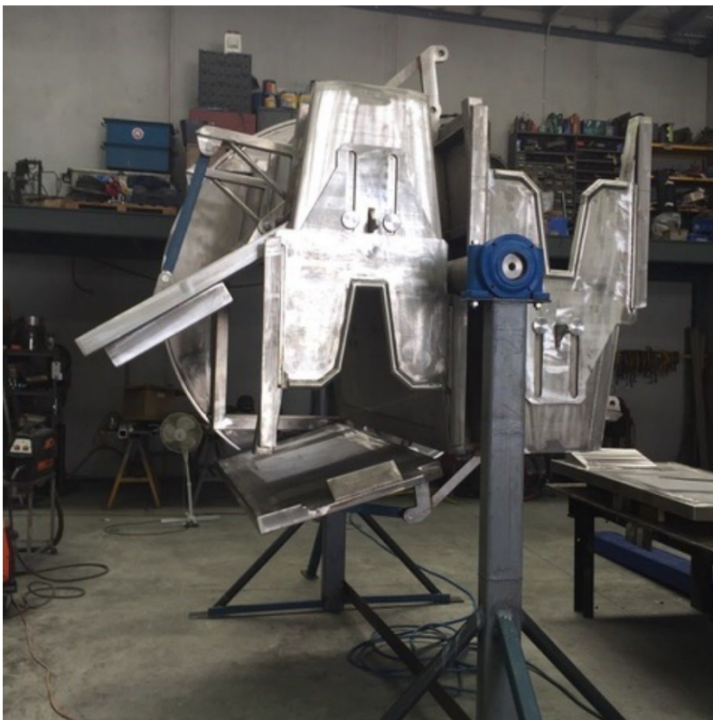
Figure 5: View of the neck capture, side and 'top' doors opened to allow ejection of the animals when inverted. Image taken during workshop construction. In this image, the upright side is to the right, and the inverted side to the left.
