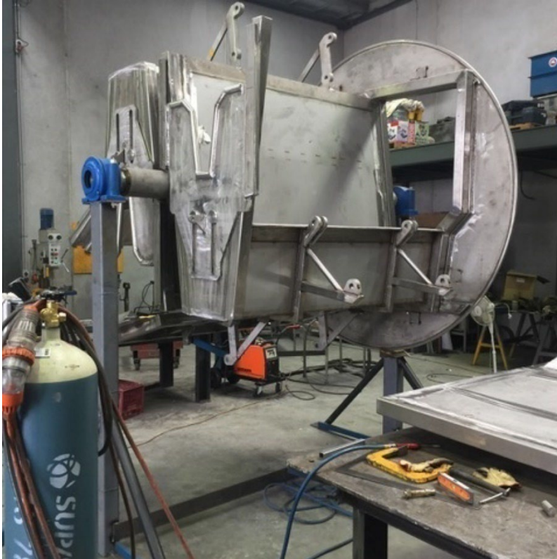
Figure 6: Side view of the upright section of the rotating restraint box. Image taken during workshop construction. In this image, the animal would be facing to the left, with the head protruding through the 'U'-shaped aperture left of middle, upper portion.
