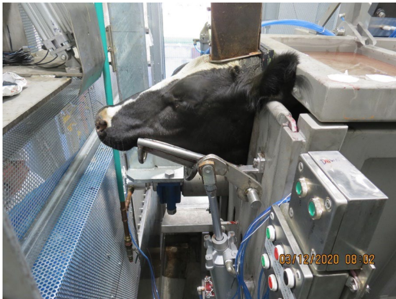
Figure 11: Animal in restraint with chin lift activated and applicator in position, immediately prior to DTS energy application.
