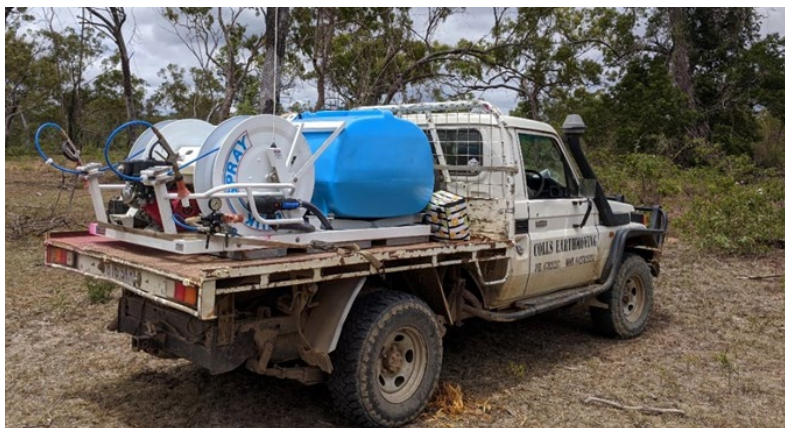
Figure 2: QuikSpray unit on Coll's Earthmoving vehicle ready for rubbervine spraying at Glenroc, Gumlu
