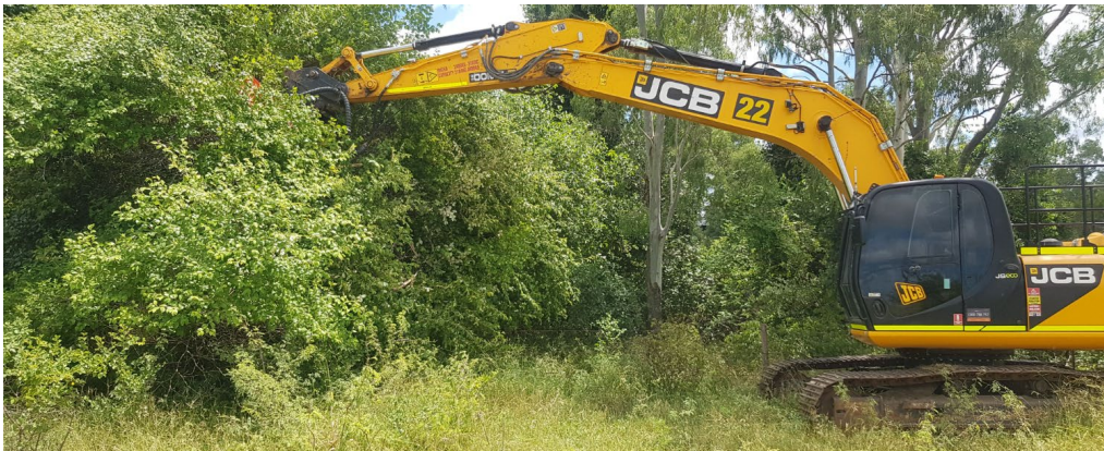
Figure 6: Utilising the Flail Mulcher to remove chinee apple, Sonoma station
