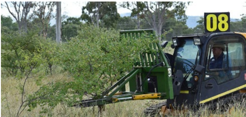
Figure 1: Bobcat mounted Auscrimper sucker puller, Glenalpine, Bowen
