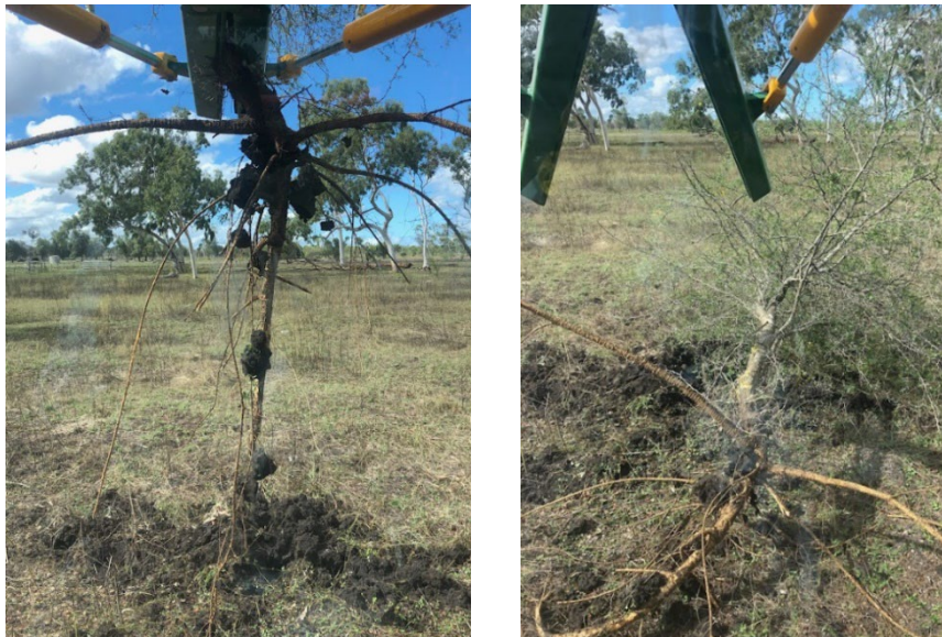
Figure 4: Auscrimper sucker puller removing prickly acacia (left) and completed (right)
