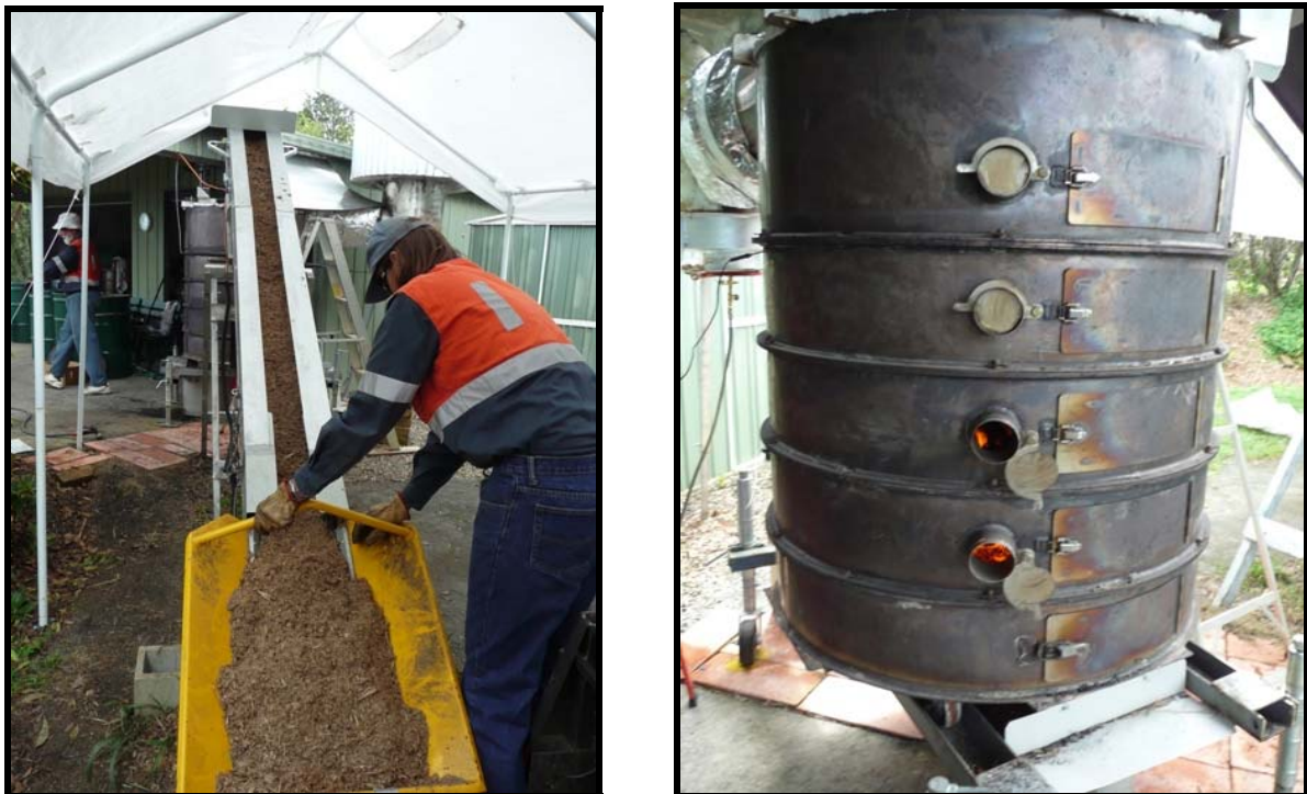
Figure 4.5: Feed conveyor on left and gasifier on right
