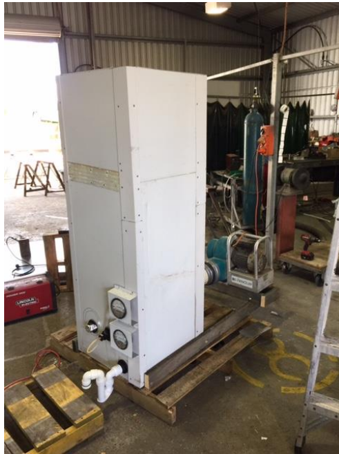
Fig 10: Test apparatus 2 m (H) x 500 x 500 mm (Internal dimensions) showing air pump, drain, pressure gauges and test port
