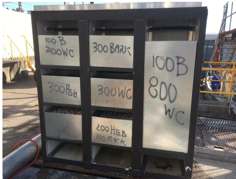
Fig 17: View of pilot Scale biofilter with cartridges (non-condensables in this image) (Note: Cell A, Tray 1, bottom left is not marked and contains 300 Hebel™)
