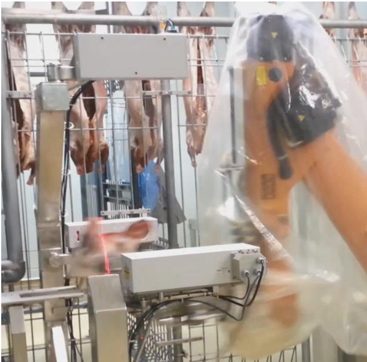
Figure 5: LEAP 5 system utilizing laser topography to determine product shape and the ideal cutting locations
