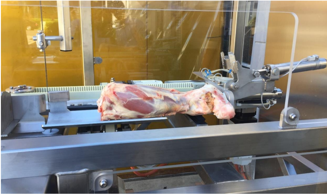
Figure 3: Beef Heavy Bone Saw with product loaded ready for processing during factory acceptance trials
