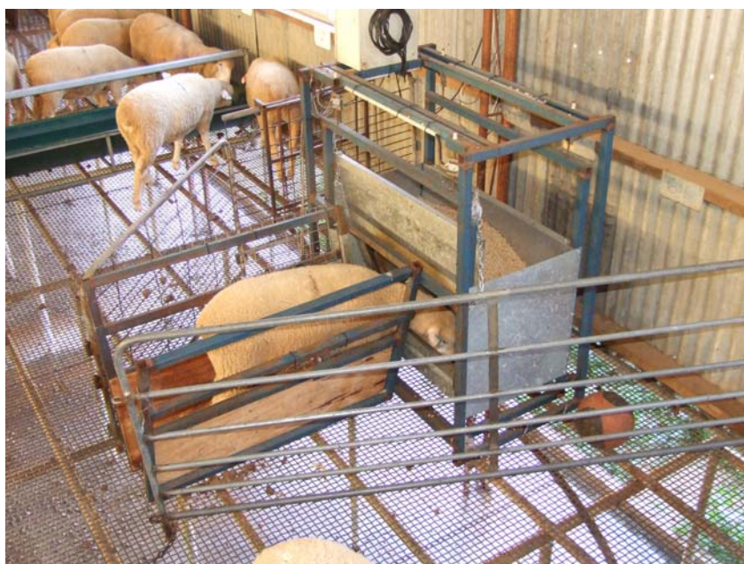
Figure 1. Lamb eating at automatic feed intake unit, showing V race, exclusion zone around the feeder and suspended feed hopper, electronics are housed in the electrical box mounted on top of feeder (with cable looped on its back).
