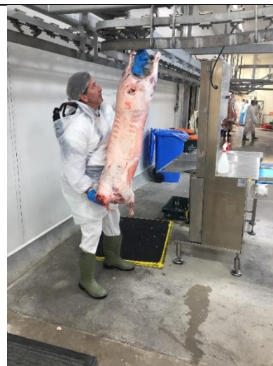
Image 2: Overhead lift of carcass with the V3 shoulderX.
