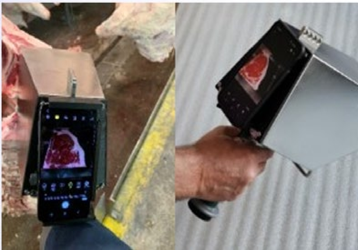
Figure 1. E+V beef grading VBG Smart camera unit similar to the one commissioned at Teys trial site.
