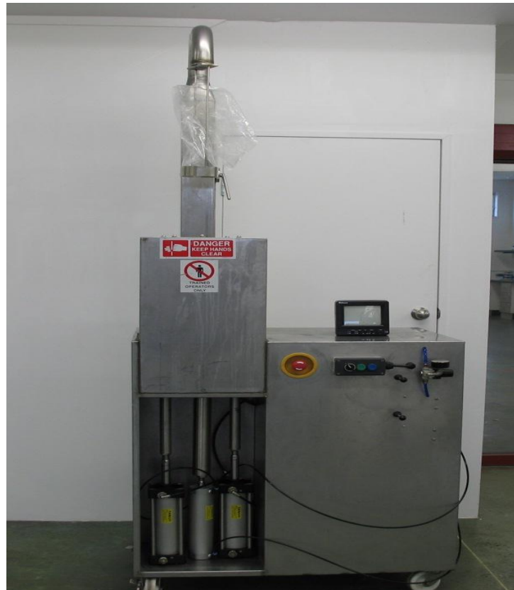
Figure 3 – Meat stretcher prototype with a frame constructed to hold the packaging at the mouth of the Boa (ie stretching component).
