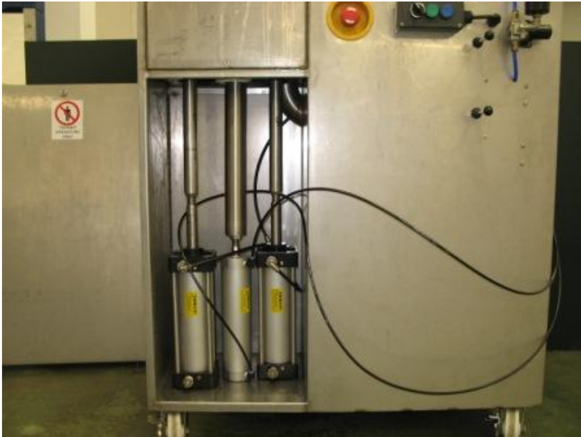
Figure 5 – Meat stretcher prototype with additional pneumatic ram has been inserted from below the Boa, which extends into the product compartment of the sleeve.
