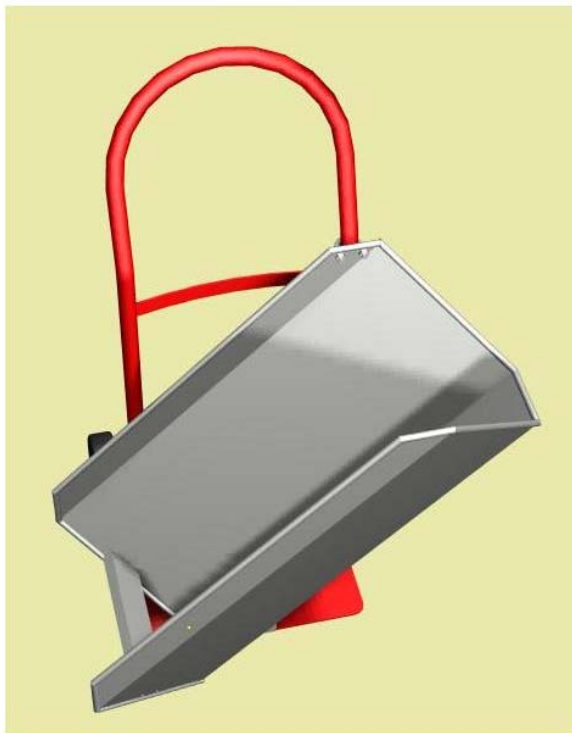
Figure 2: Final trolley prototype (above figures are JPEGs developed from the AutoCAD drawings).
