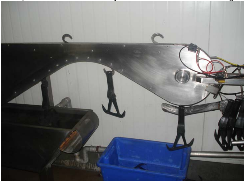
Image 31: The Skid Supply conveyor transfers skids from the skid room to the Processing Floor
