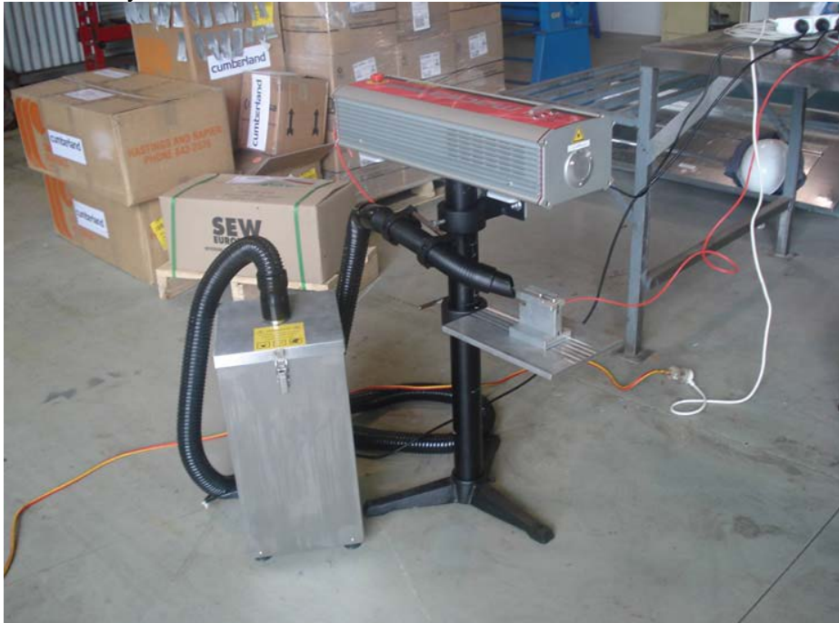
Image 1: MACSA Laser mounted on stand with fume extraction system alongside
