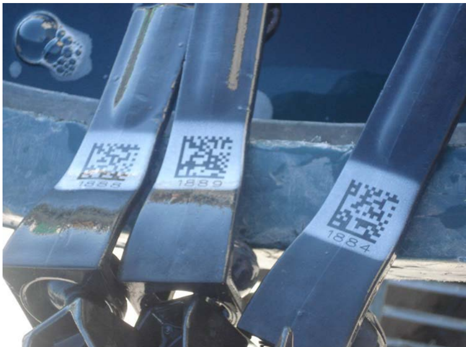
Image 29: Skids with High Strength patches being tested in the soak tubs
