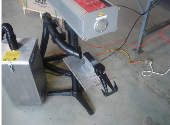
Image 3: Laser is ready to print with skid sitting in the cradle
