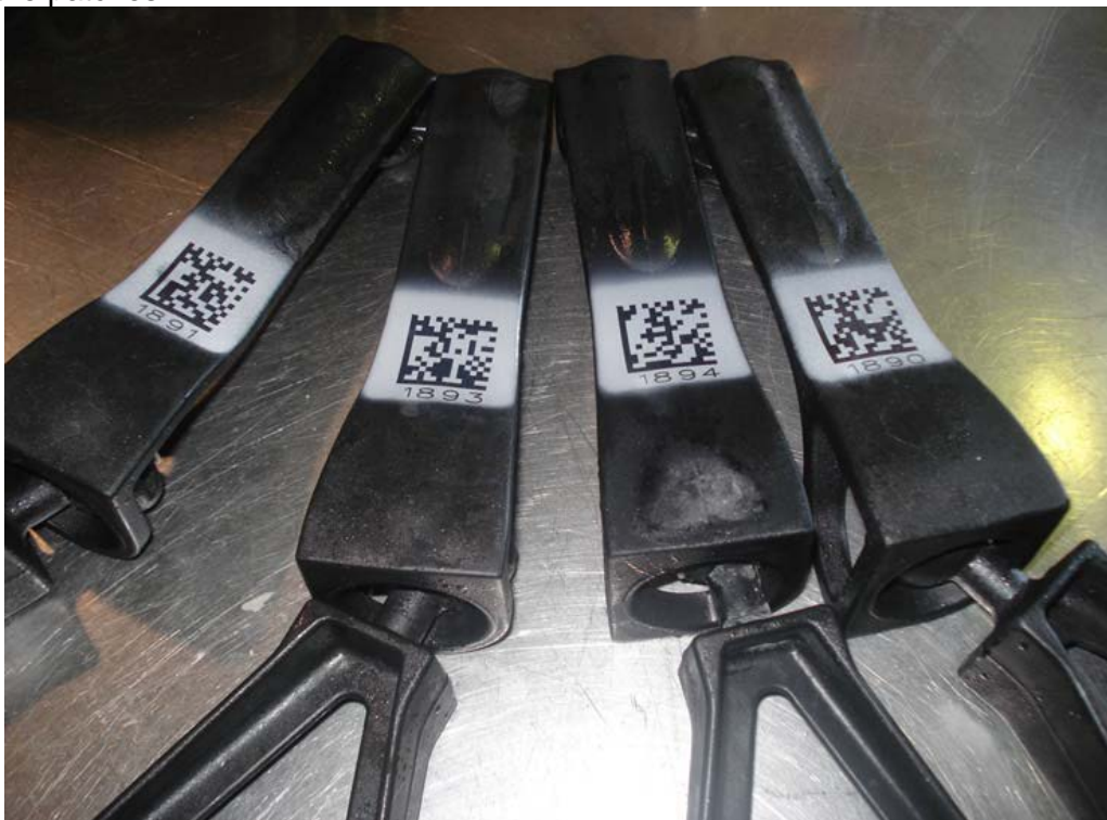
Image 24: Two skids with each type of patch were subjected to 48 hrs at -20 deg C, note the ice on the skids
