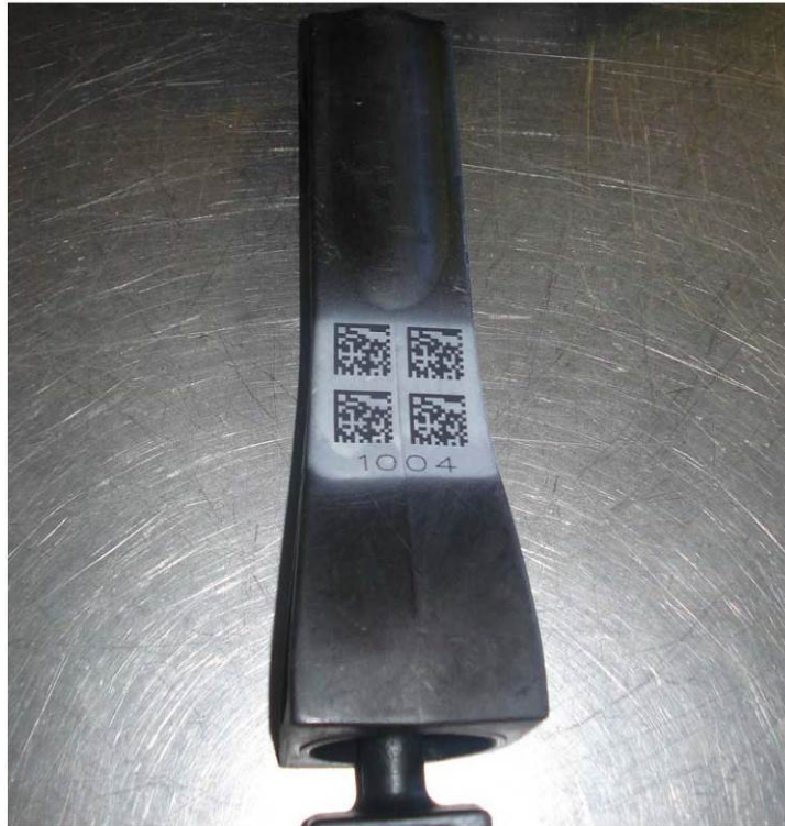
Image 9: Skid with barcode printed four times
