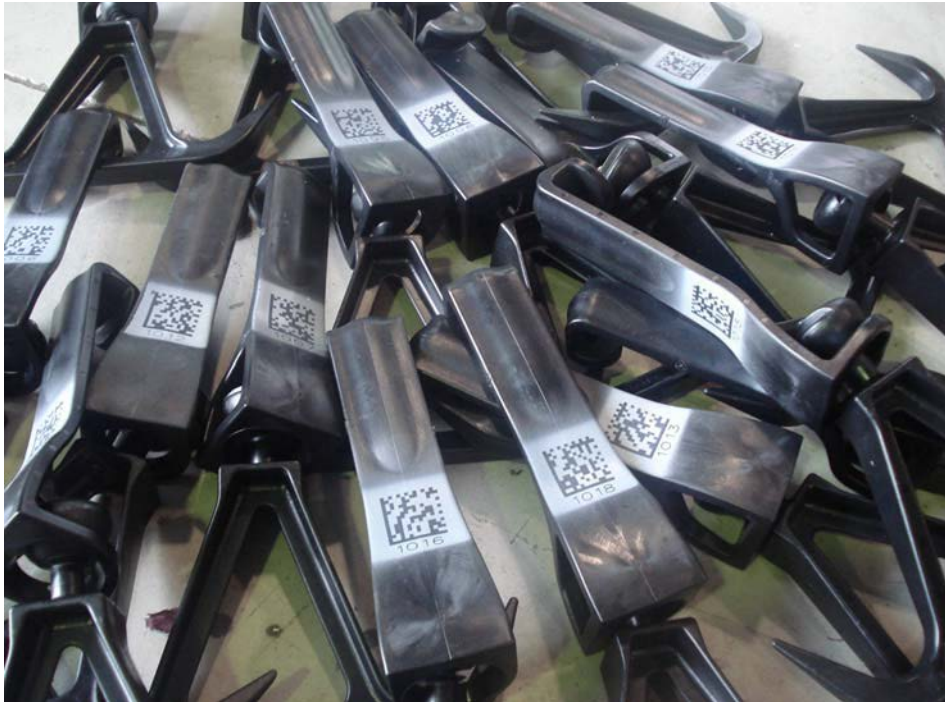
Image 5: Skids with patch and Data Matrix barcode and matching sequential number The completed skids were then placed in boxes ready for use.
