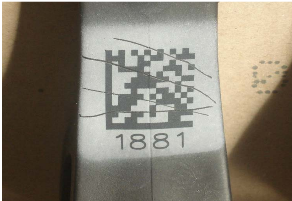
Image 22: Skid 1881 with barcode damage, reads okay.
