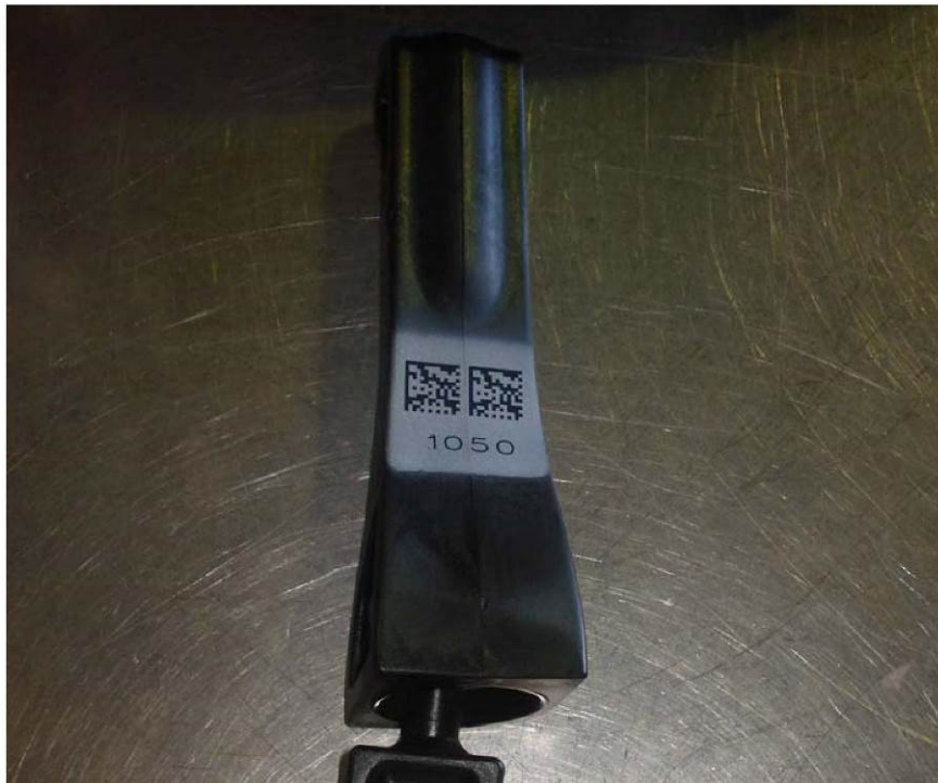
Image 8: Skid with barcode printed twice
