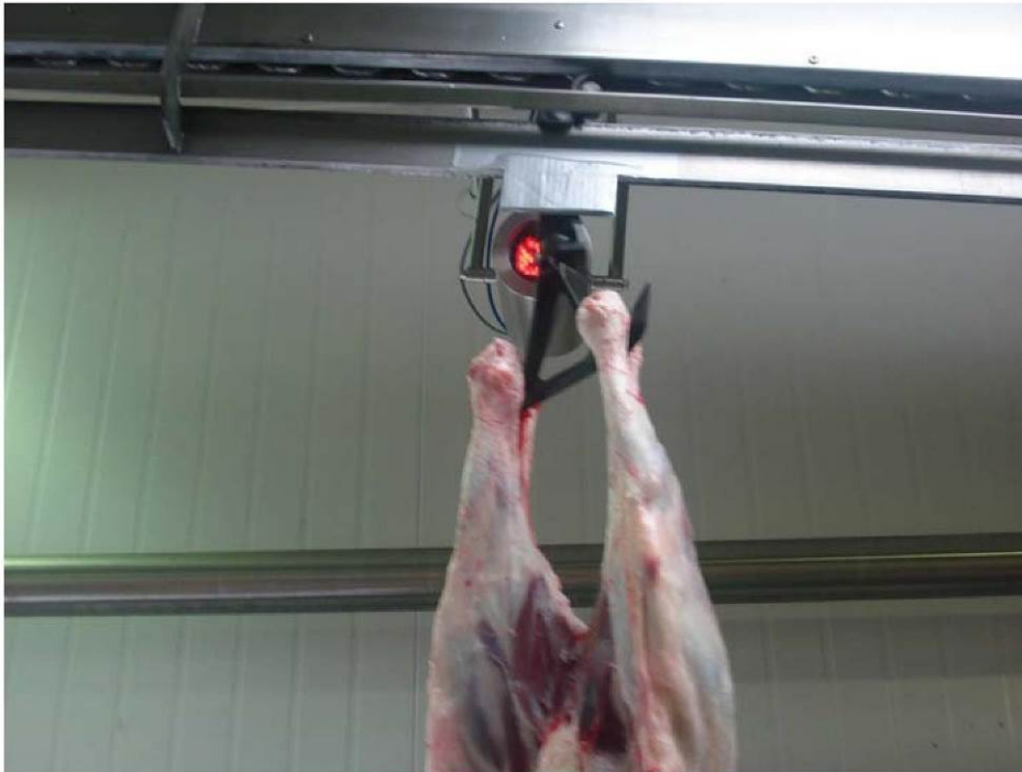
Figure 2: camera has been triggered and the LEDs are illuminated
