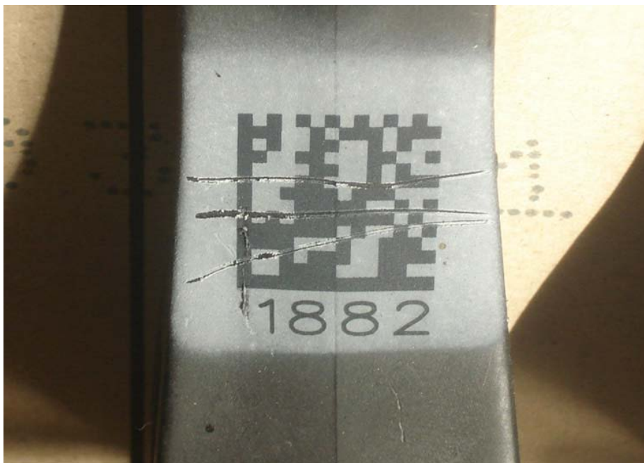
Image 19: Skid 1882 with barcode damage, reads okay
