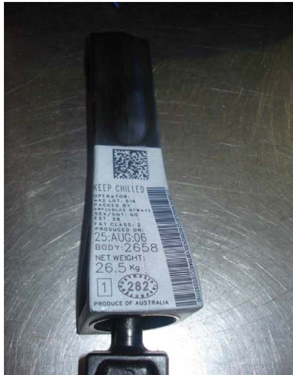
Image 32: Skid printed with the carcass ticket data and an additional Data Matrix barcode
