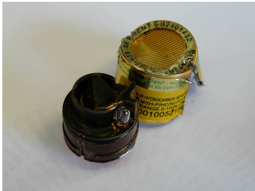
Figure 7. Infra-red Dynament® methane gas sensor contamination
