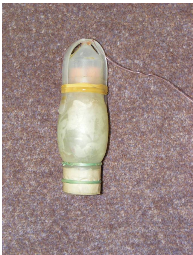
Figure 6. Diffusion cell made from a controlled release device (CRD) and a polydimethyl siloxane membrane
