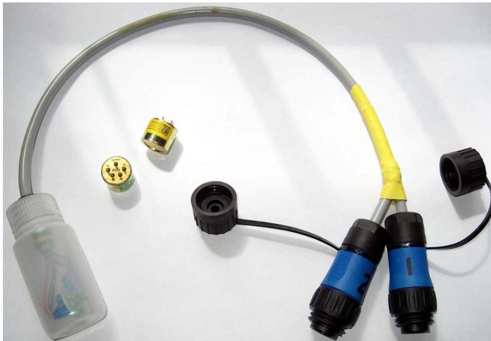
Figure 1. Early intra-ruminal device incorporating 2 gas sensors housed in a sealed low density polyethylene Nalgene® container. Gas diffusion across the plastic proved to be slow with a long lag time to reach equilibrium. The system was very labour intensive as fistulated animals had to be yarded to collect rumen gas concentrations in real-time.
