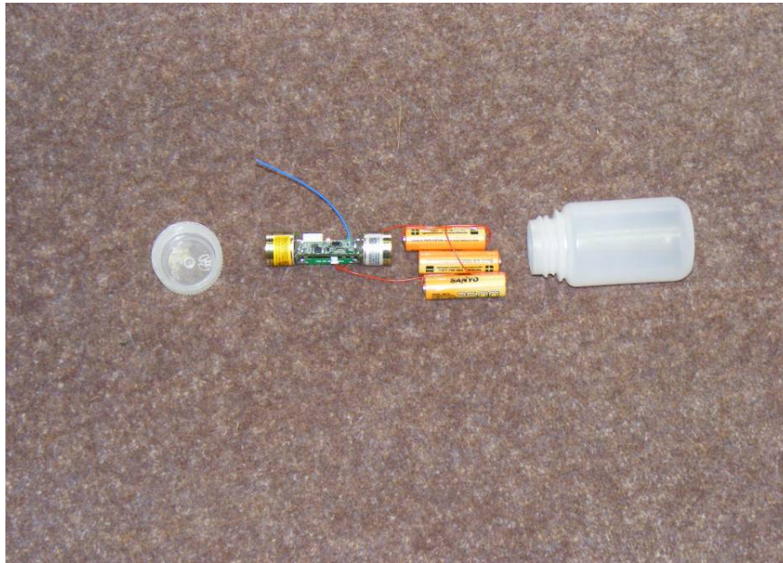
Figure 3. Intra-rumen sensor unit, batteries and polyethylene plastic container
