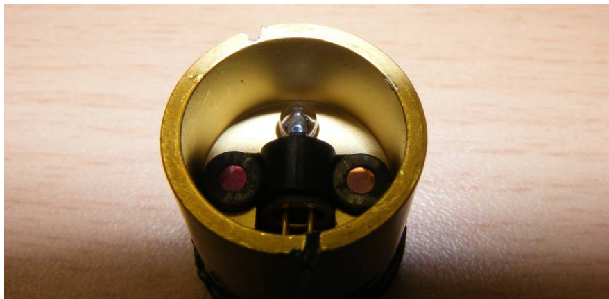
Figure 9. Dual E2v® gas sensor with the top removed showing small contamination on the photodiodes after it was placed inside the diffusion cell and installed in a rumen.
