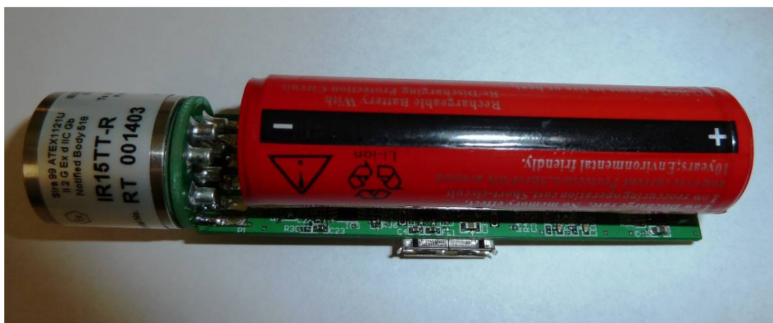
Figure 13. PACP Serqet wireless Intra-rumen sensor unit
