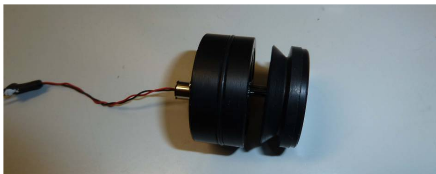
Figure 10. Gas cut-off valve with small electric motor
