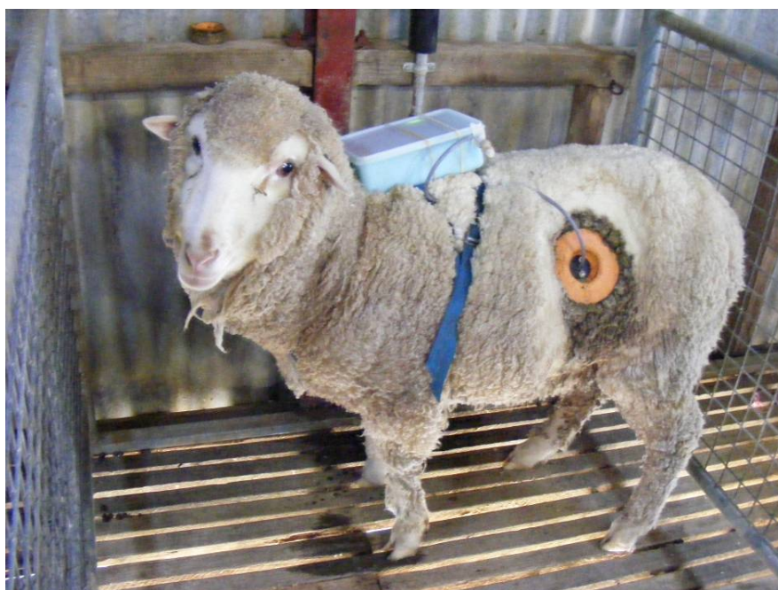
Figure 12. e2v® intra-rumen gas testing assembly on a rumen fistulated sheep
