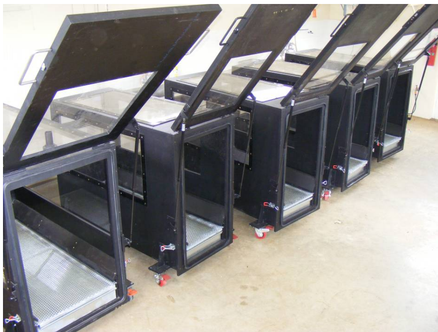
Figure 17. Open respiration chambers at F D McMaster Laboratory
