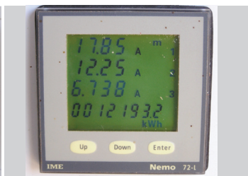
Figure 5: IME Nemo 72-L power monitor
