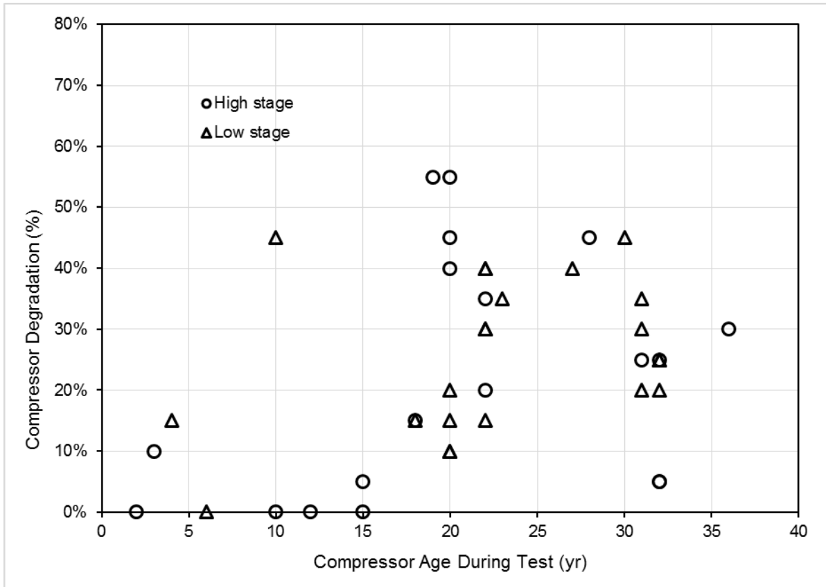
Figure 7 Compressor degradation versus compressor age for high stage and low stage units.
