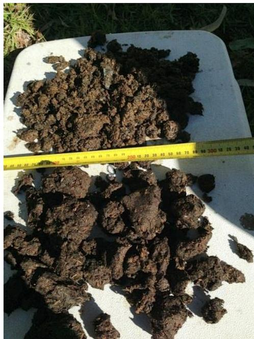
**Photograph 50 – Particle sizes of freshly scraped pen manure from feedlot 3 before (bottom) and after (top) the pre-treatment**
