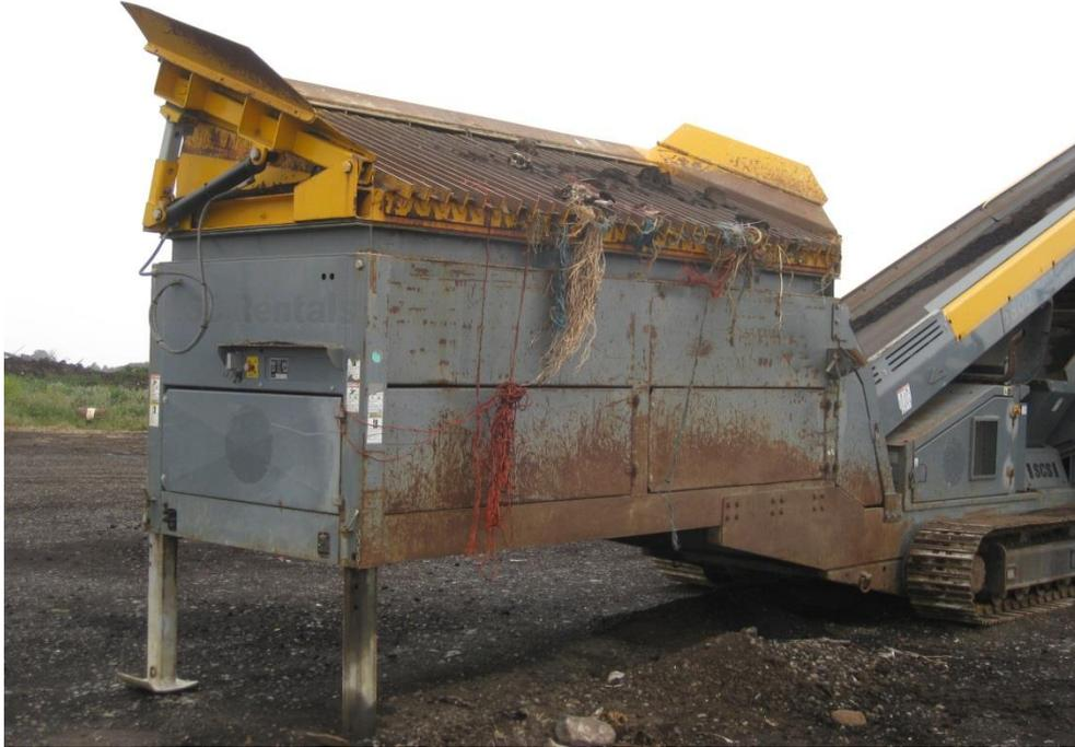
**Photograph 14 - Intake bin to manure screening plant showing baling twine**
