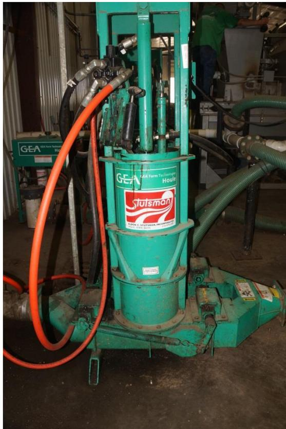
Photograph 63 – Positive displacement slurry pumps
