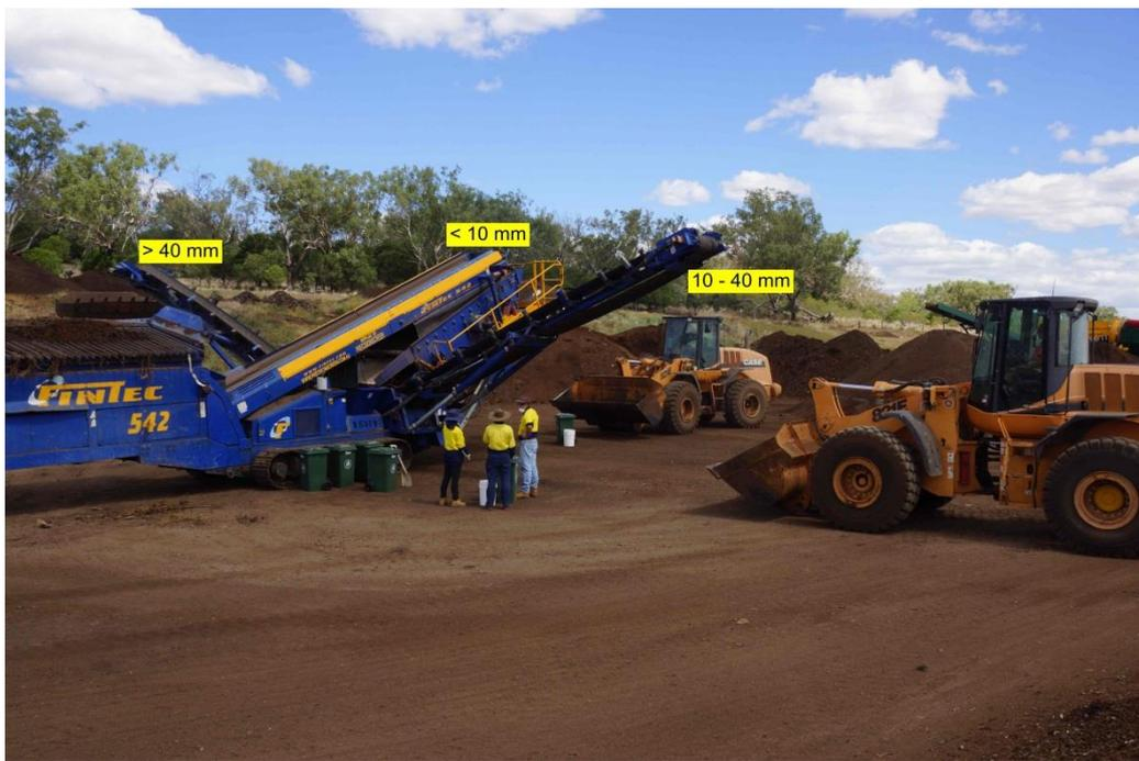
Photograph 56 – Three-way vibrating screen
