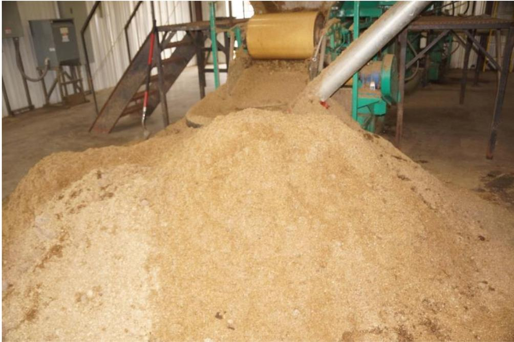
**Photograph 27 – Separated solids from digester effluent**
