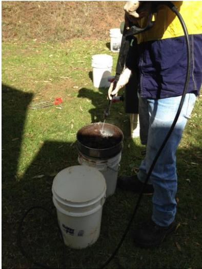
**Photograph 48 – Operation of the pressure cleaner to break up manure clods**
