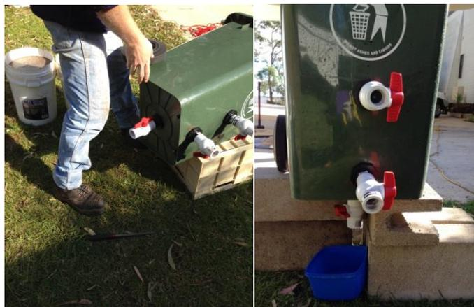
**Photograph 49 – Positioning of the three sample valves**
