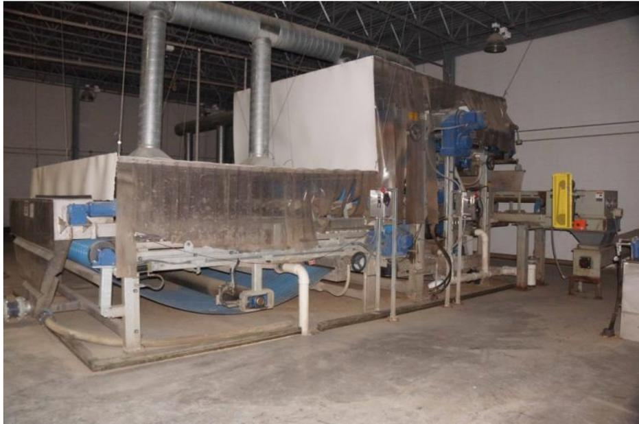
**Photograph 37 – Belt press for effluent dewatering (not operating)**
