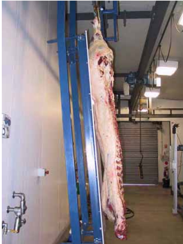
Figure 4.3 Side of beef is restrained on a 'stabilisation' board
