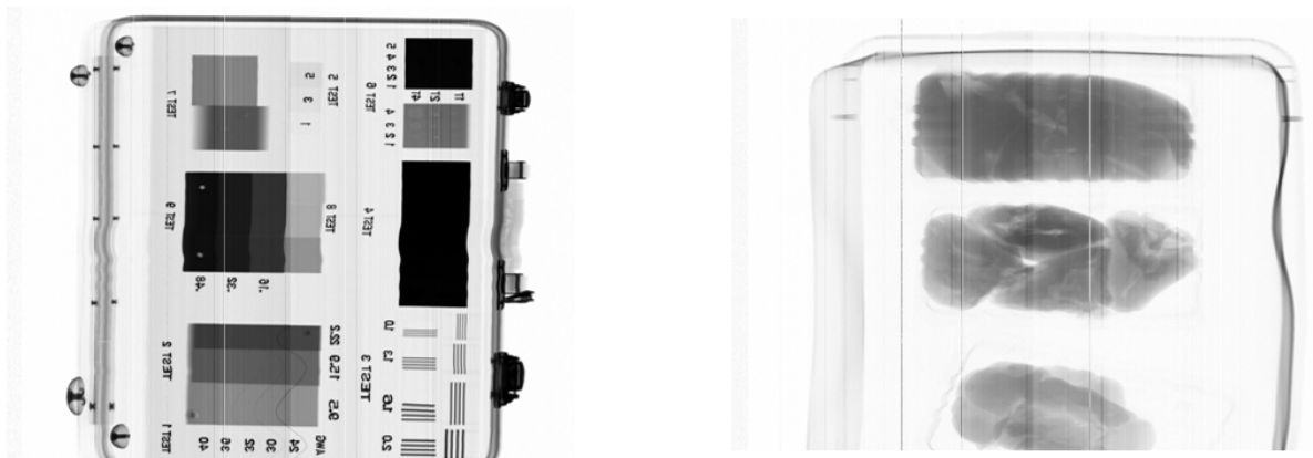
Figure 4: Multi-energy X-ray image data – central up-shooter view. Left: X-ray image quality test piece. Right: Beef offal.
