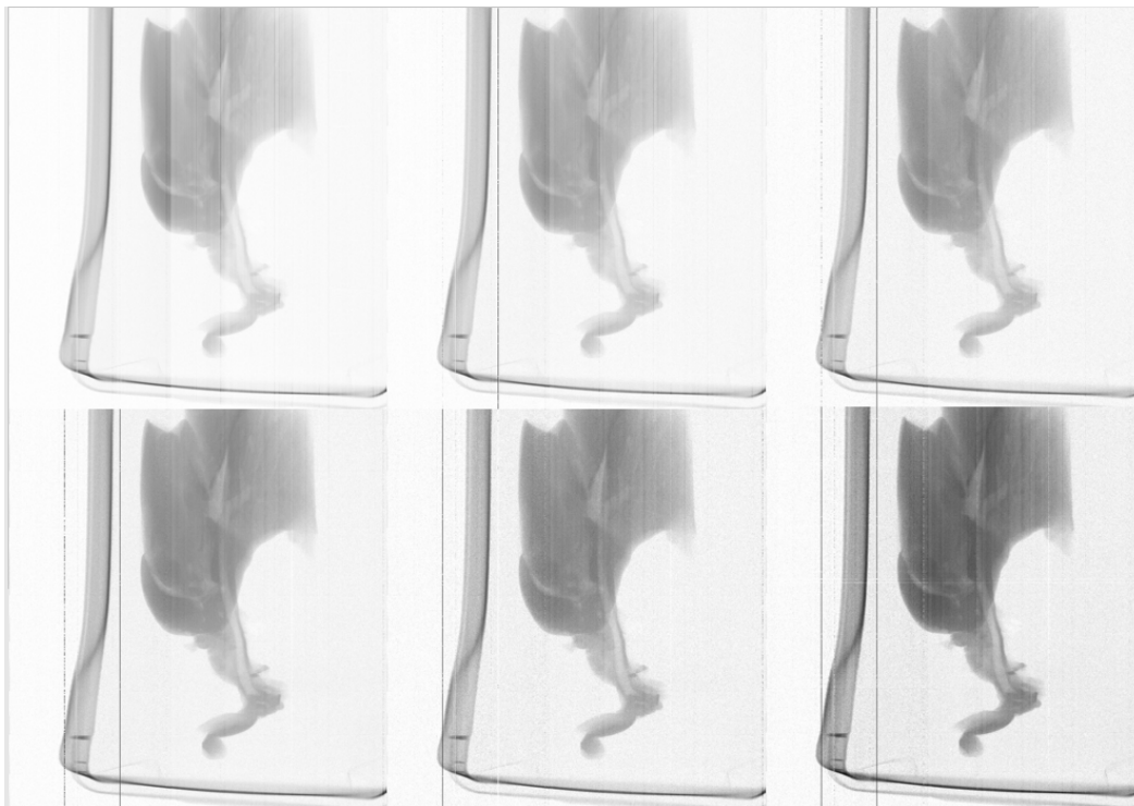
Figure 24: Multi-energy X-ray scan of lamb lungs shown at varying greyscale contrast.
