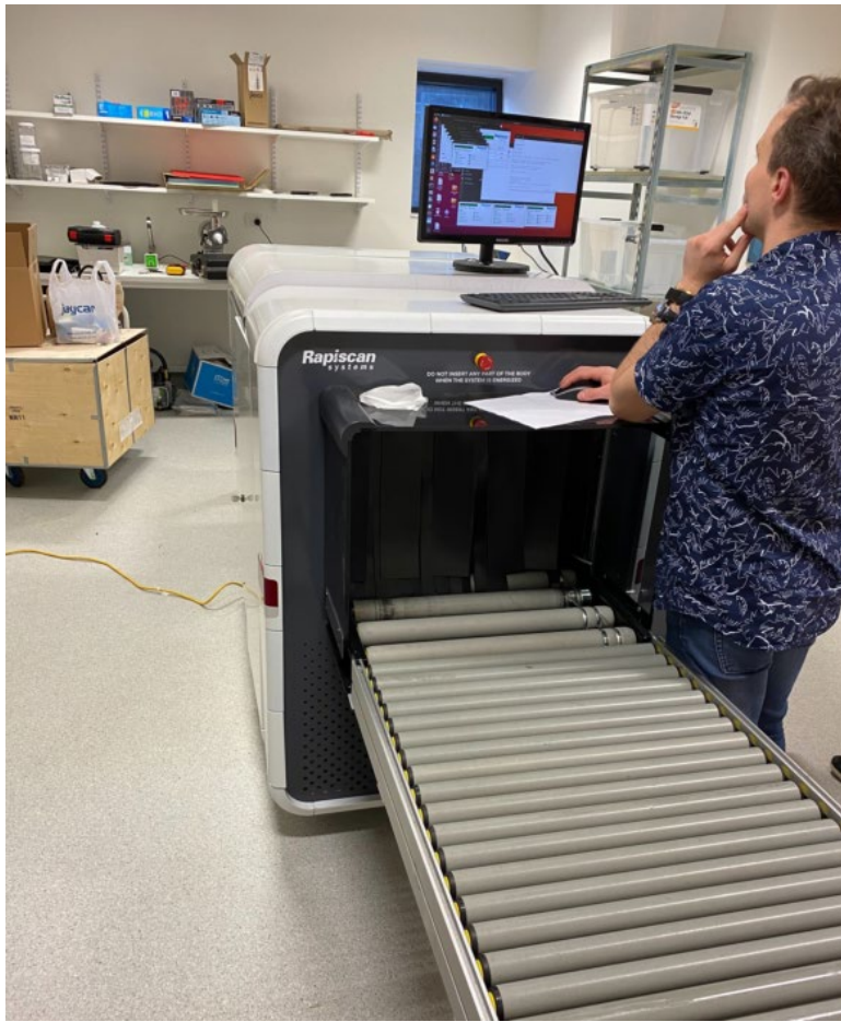
Figure 11: Photograph of the installed multi-sensor system showing the passive roller bed onto which samples are placed in trays prior to X-ray scanning.
