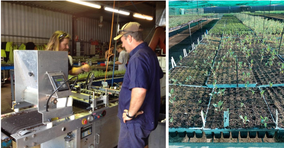
Fig. 4.37. Using a mechanised planter to sow naked and coated seeds at Chatfields Tree Nursery in Tammin (Dustin McCreery and Matt Wilmot pictured).
