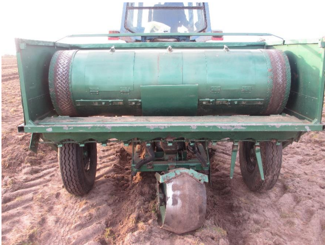
Fig. 4.26. Niche seeding machine from Cranbrook (Walsh and Lehmann families).
