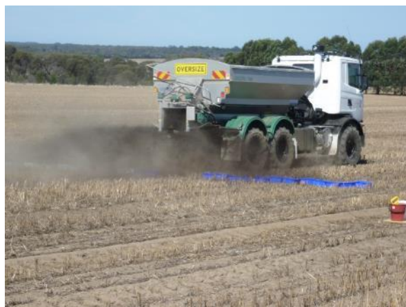
5.9) Calibrating a truck spreader at Freshwater Creek
