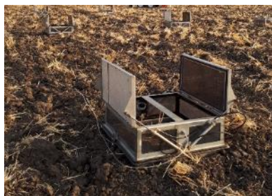
5.5) Automated chamber in wheat stubble at Felton
