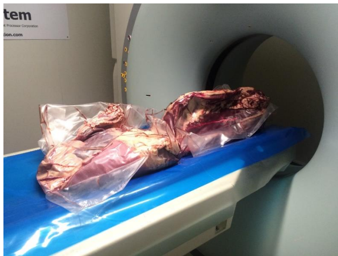
Figure 4: Vacuum packed "primals" being CT scanned
