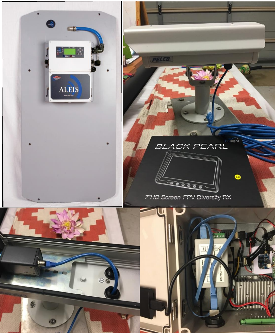
Fig. 12. Components of the automated prototype to detect and draft animals with high body temperature. A) RFID system, b) IRT camera system.
