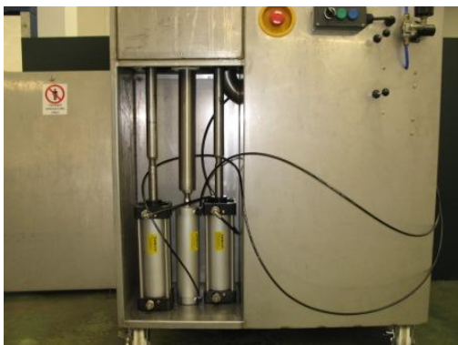
Figure 2. Pneumatic ram has been inserted from below the boa, which extends into the product compartment of the sleeve
