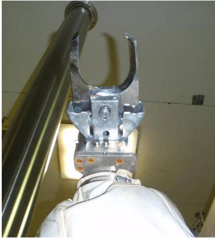
Fig. 15 Rear Hock Tipping Tool installed on site
