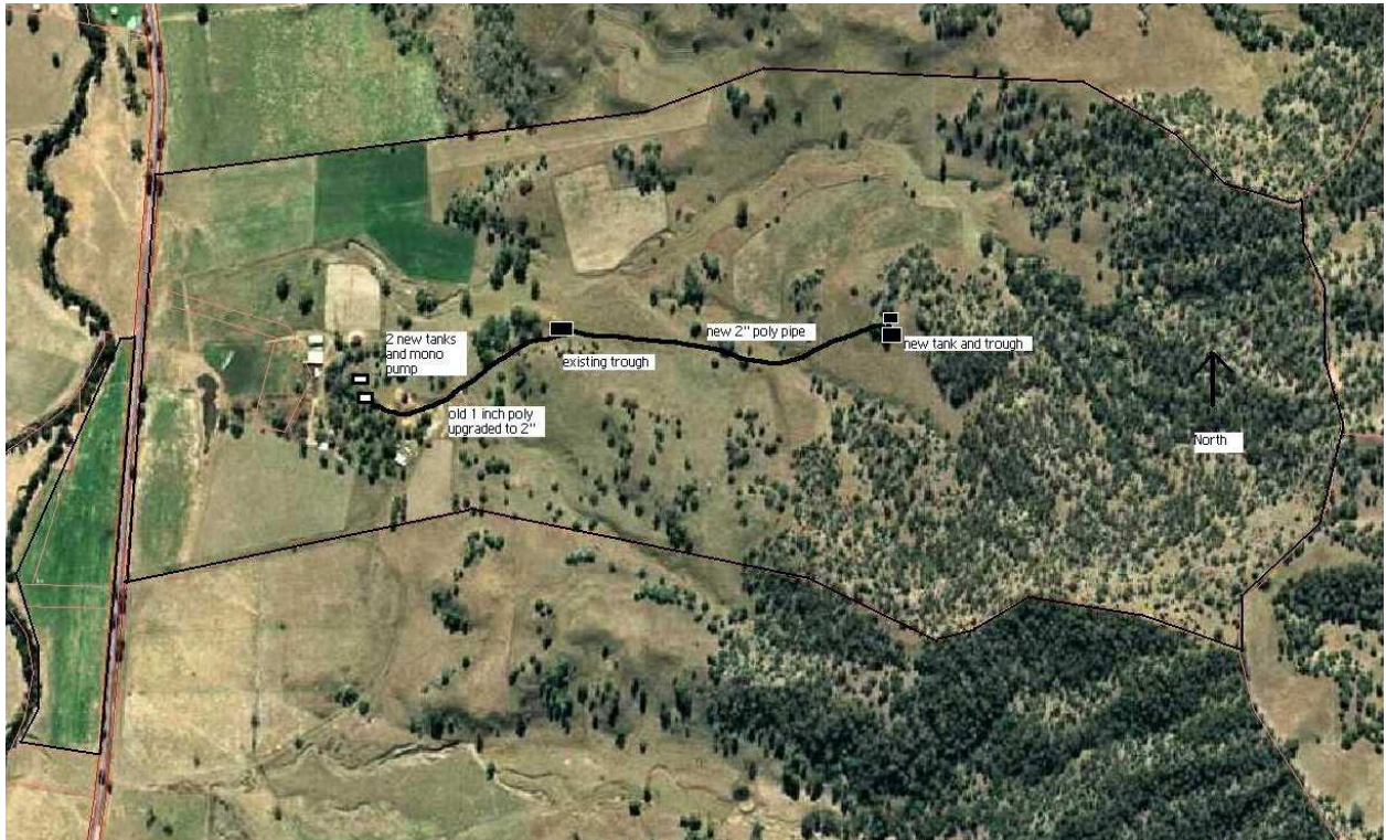
Aerial photo showing location of new infrastructure
