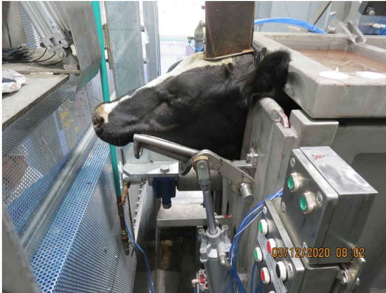
Figure 6: An animal in position, prior to DTS application, with the chin lift applied and the waveguide applicator in position on the forehead. The door allowing access to the inverted stunned animal is now closed.
