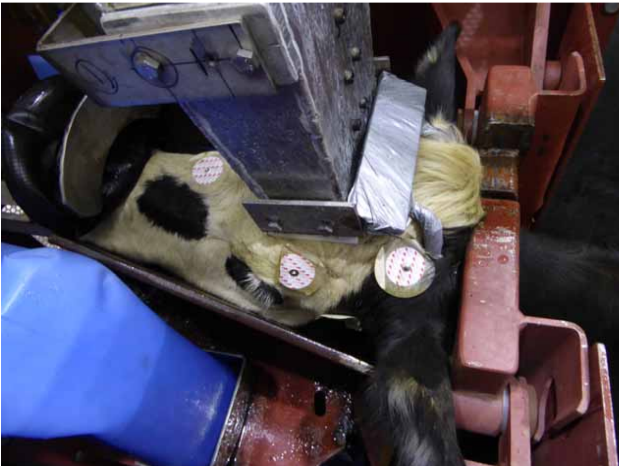
Figure 2: Waveguide positioned on forehead of animal. White disks are EEG recording pads, blue container is a water reservoir for absorption of stray energy, nose 'comforter' has a cushioned contact area.
