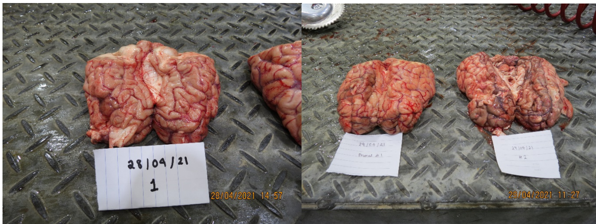
Figure 3: Brains from three cattle processed using DTS. Left 180 kJ; middle 180 kJ; right 320 kJ. Destruction of the brain tissue of the frontal lobe can be seen in the sample on the right, and the brain does not maintain its form when placed on the bench. In the samples at middle and left, the brains maintain their form, and the tissue structure is intact.
