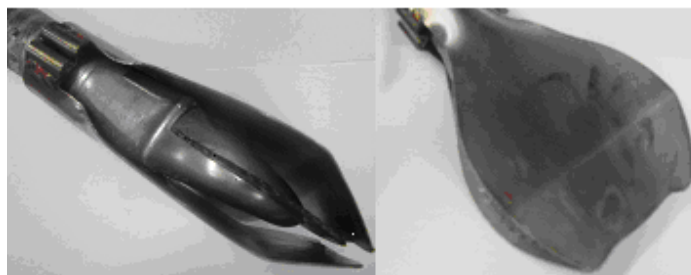
Fig. 3 Reciprocating Blade Tool
