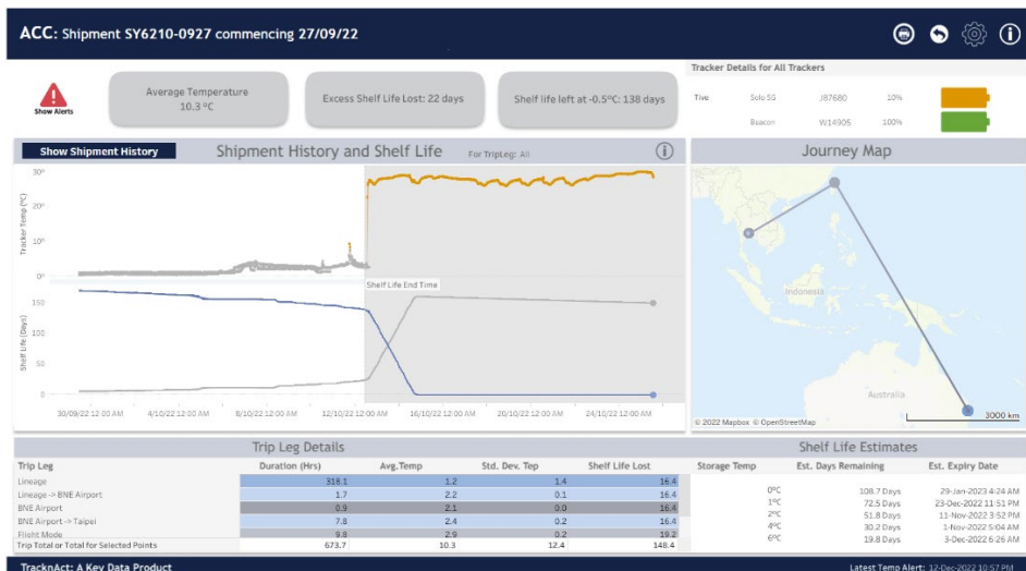
Figure 4a Consignment Report (Shipment end date and Shelf-Life impact calculation separated by leg destination)
