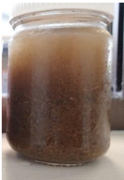
Photo 7: Aerobic Sludge Sample
