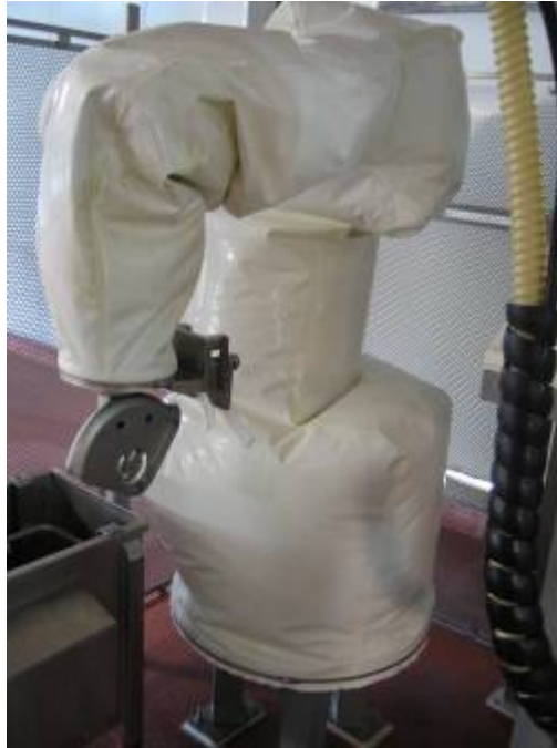
Fig.1 Brisket Saw installed at GMP (shown without blade attached)
