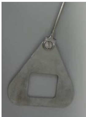
Figure 1: Shear blade for the modified WB shear force device, showing the square hole in the blade.
