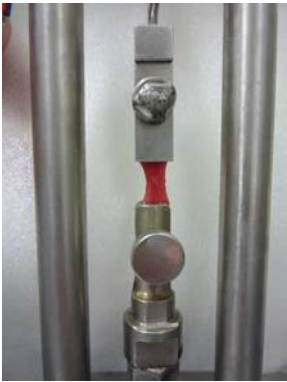
Figure 6: Meat sample held between serrated jaws for HIT measurement.
