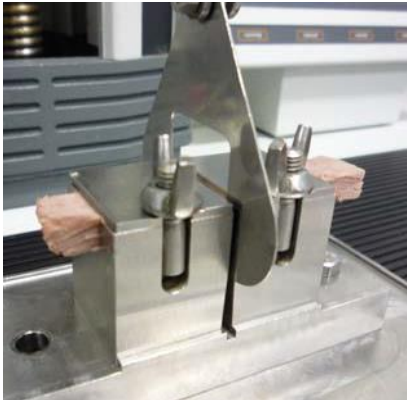
Figure 3: Modified WB shear force device.
