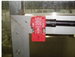
Cell access door safety Switch
