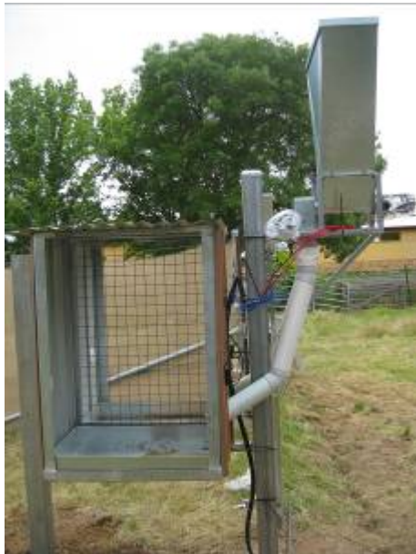
Fig 2a Feeder and hopper
