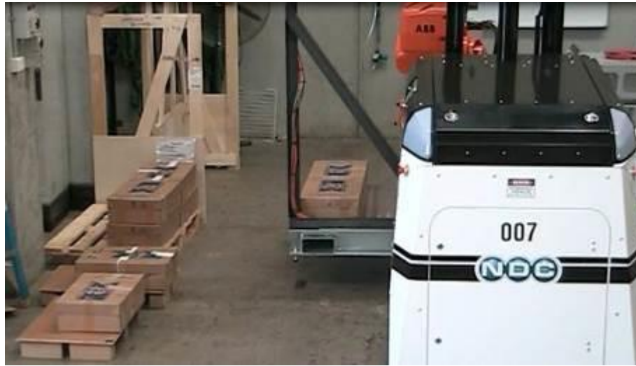
Fig 28. This image shows the Pallets and cartons loaded onto the robot platform for the Mixed Pallet and order picking demonstration.
