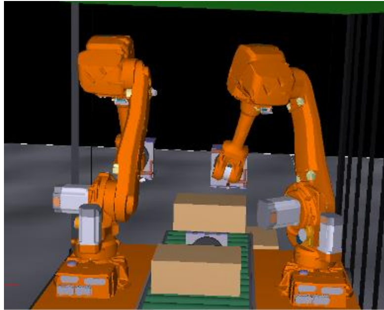
Fig.15 Concept V4 – Dual Robots with pneumatic pop up for carton pickup and MAR patented translating grippers for carton placement
