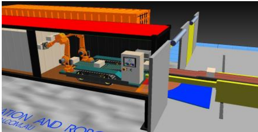
Fig.29 Final concept design featuring telescopic conveyor
