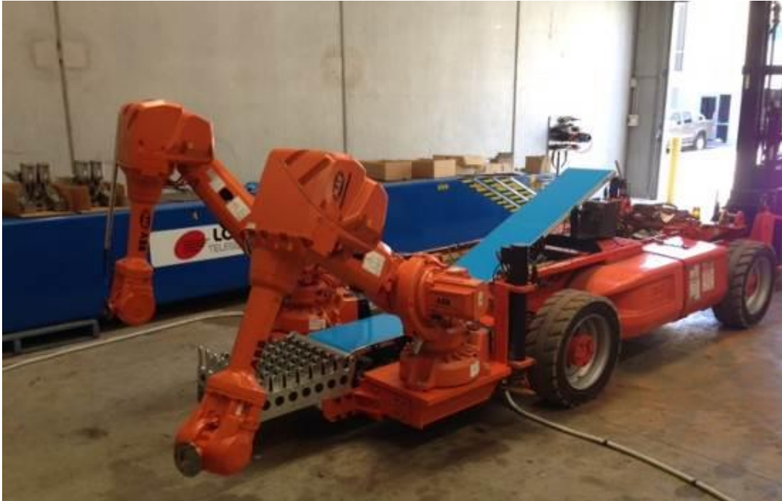
Fig.37 Vehicle Robots mounted, retrofitted conveyor and pick off station in place
