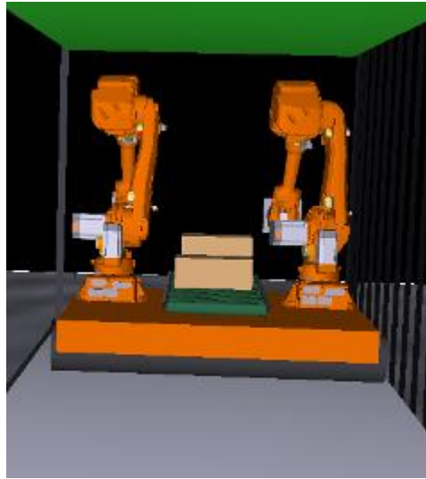
Fig.13 Concept V3 – Dual Robots with pneumatic pop up for carton pickup
