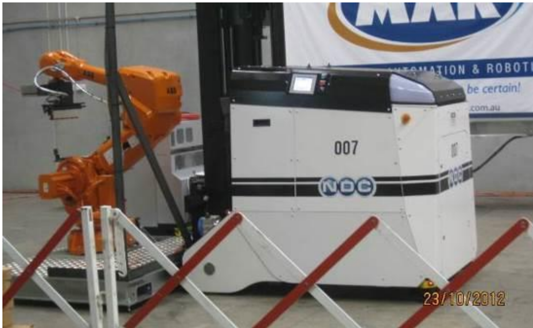
Fig. 24 Image showing AGV, platform, robot and gripper
