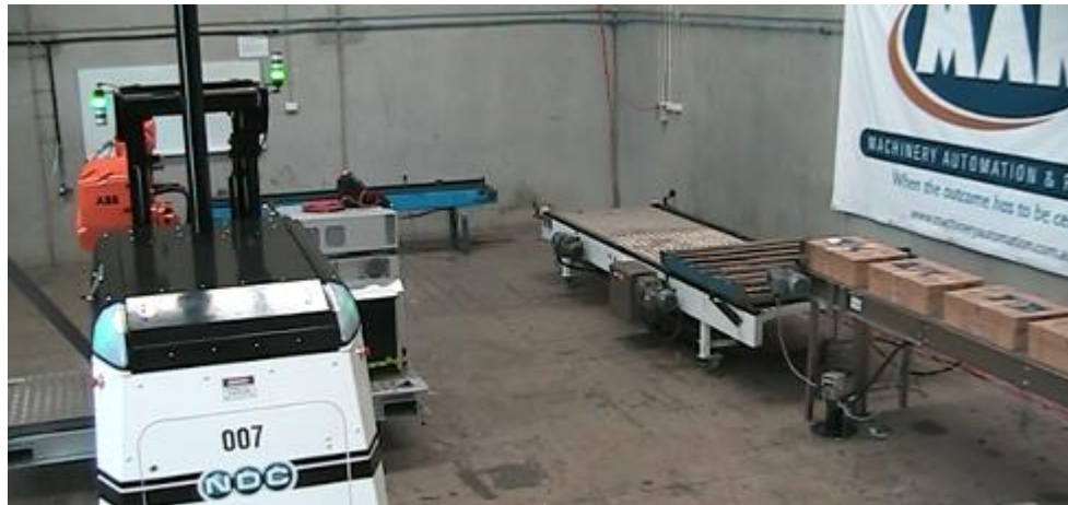
Fig 25 This image shows the infeed carton conveyor, and the palletising and de palletising conveyors
