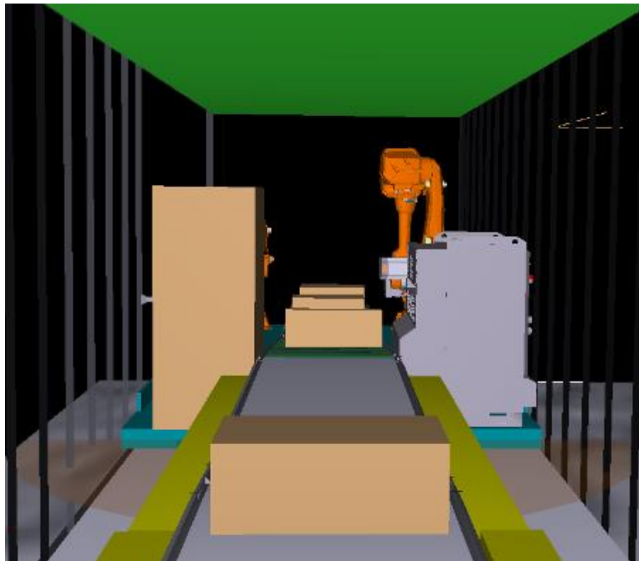
Fig.18 Concept V5 – Track vehicle with robots mounted on the front and electrical panel and robot controller at the rear
