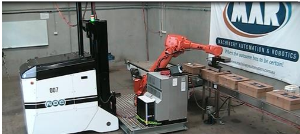
Fig. 26 Image shows the system palletising from the infeed conveyor
