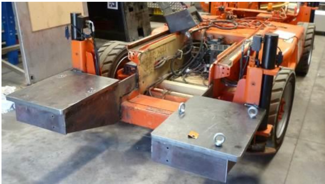
Fig.36 Plates fitted to front of vehicle to allow mounting of robots
