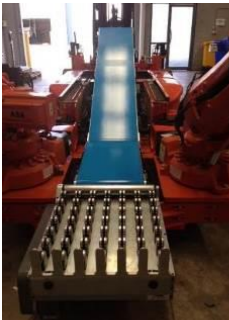
Fig.38 Retrofitted conveyor and pick off station
