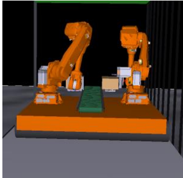
Fig.11 Concept V2 – Dual Robots with side pickup platform for pickup of cartons on short and long face
