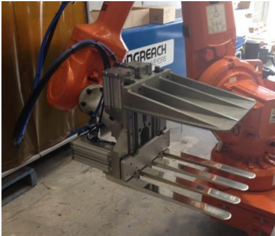
Fig.39 Carton Gripper showing pneumatics plumbed and wired
