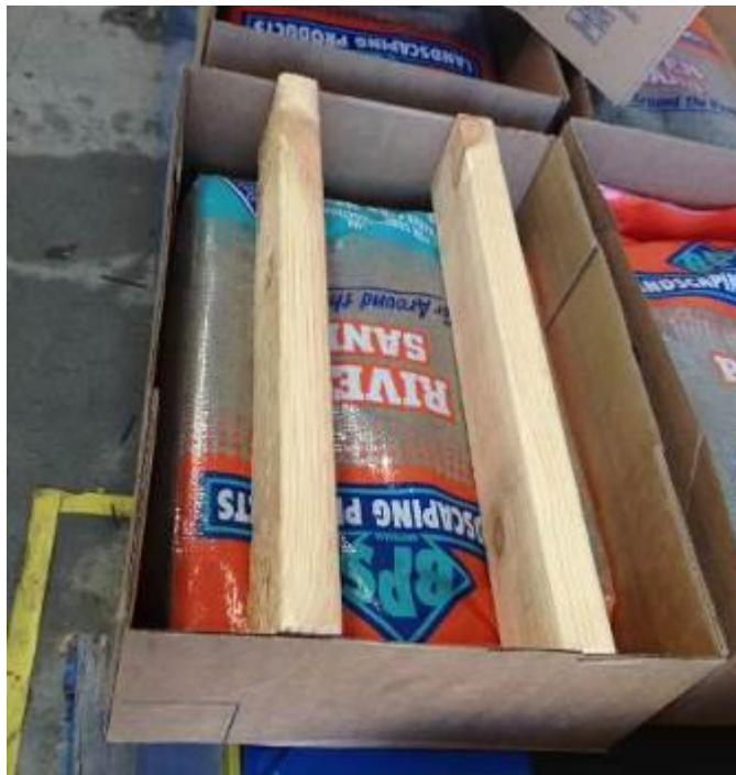
Fig.45 Cartons filled with Sand bags and wooden blocks to simulate weight and maintain form.
