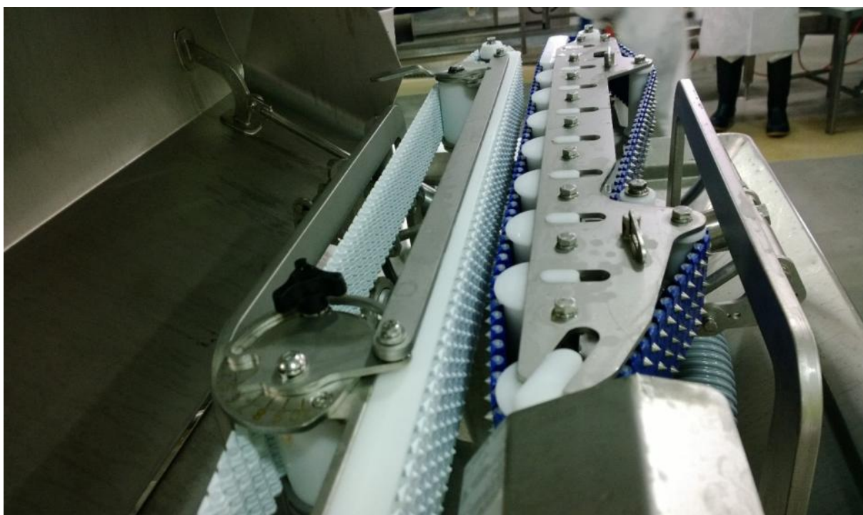
Figure 6: iFRENCH belt width adjustment mechanism
