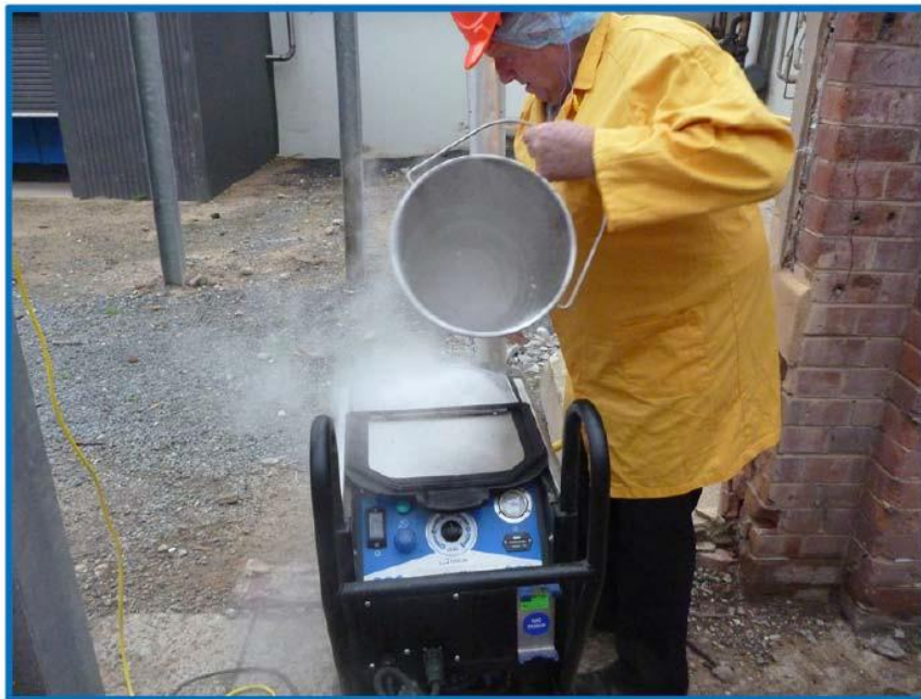
Figure 9: Filling the Blasting unit with CO 2 pellets
