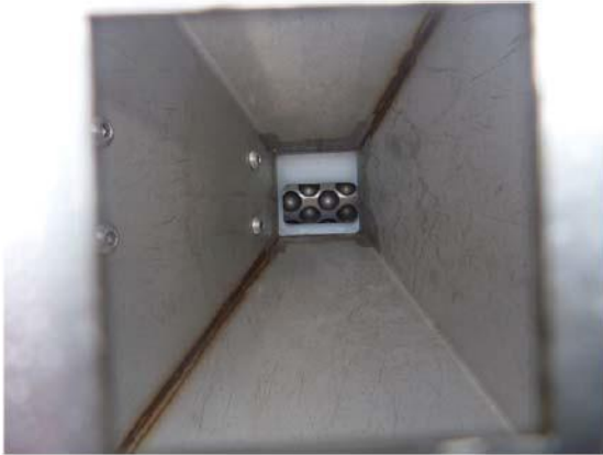
Figure 18: Blaster CO 2 metering barrel (view is looking into the top of the hopper)
