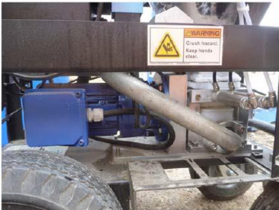
Figure 20: Motor and discharge air pipe from chamber
