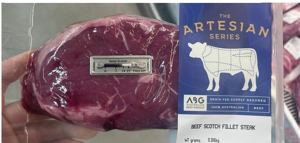
Figure 1 – Keep-It Indicator showing less than 14 days until expiry.
