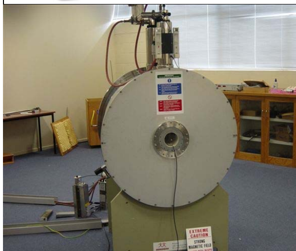
Figure 9. High Field NMR device with superconducting magnets. It is great for detailed studies but impractical for large meat samples
