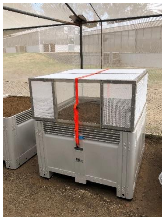
Figure 2. Completed cages, left: welded aluminium angle frame, with a polycarbonate access door, clad in white shade cloth, right: cages covered with a piece of white shade cloth, fastened to cages by bulldog clips. Image source: CSIRO
