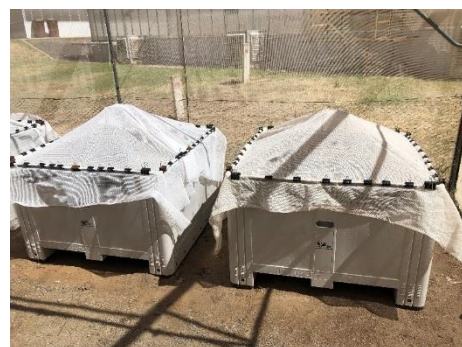
Figure 2. Completed cages, left: welded aluminium angle frame, with a polycarbonate access door, clad in white shade cloth, right: cages covered with a piece of white shade cloth, fastened to cages by bulldog clips. Image source: CSIRO
