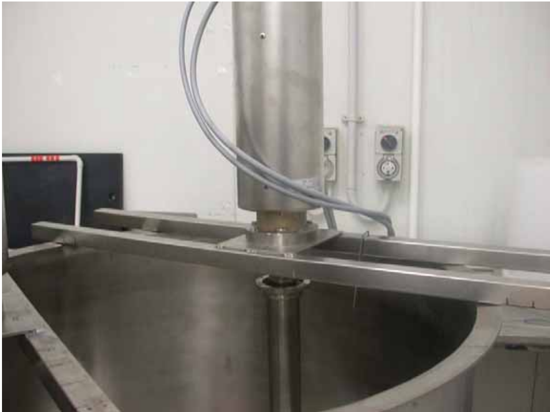
Figure 1. Sonotrode supported in original cylindrical tank.
