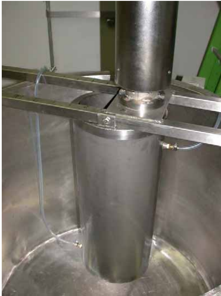
Figure 2. Ellipsoidal vessel and sonotrode supported in cylindrical tank
