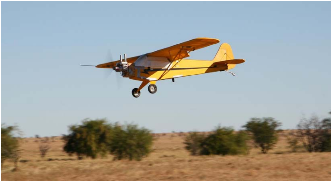
Figure A1 – J3 Cub UAV System in flight over Julia Creek, Queensland during the July 2009 flight trials. The platform and sensor payload have remained the same for the 2010 flight trials.
