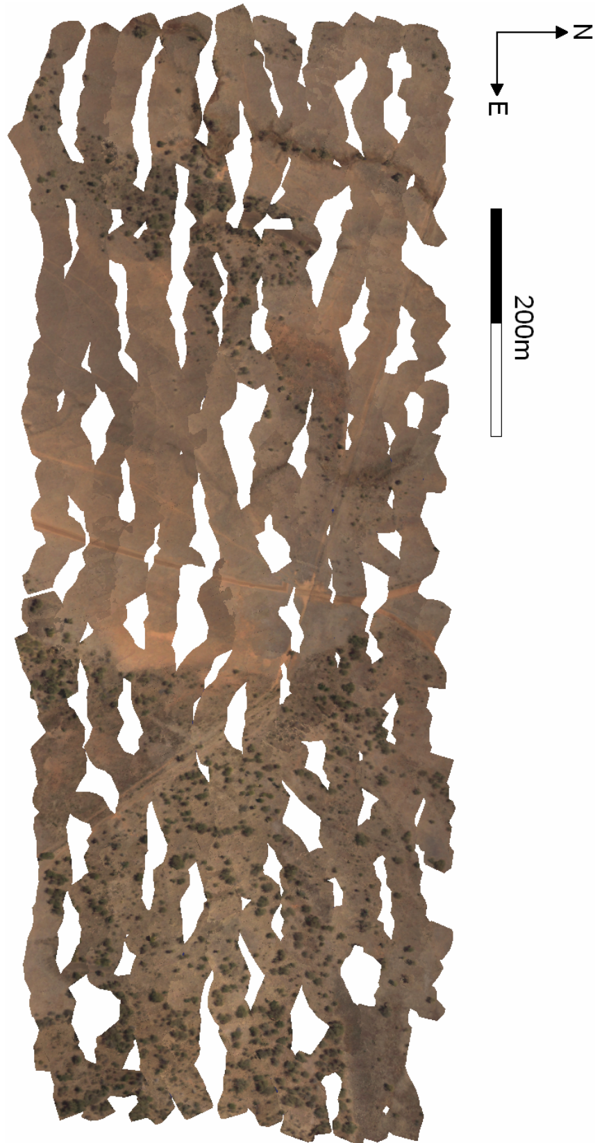
Figure A16 – Segment of constructed map of Williams Outstation from Flight 27 (gaps seen due to platform motion, future work will look at online data collection planning for improved area coverage)
