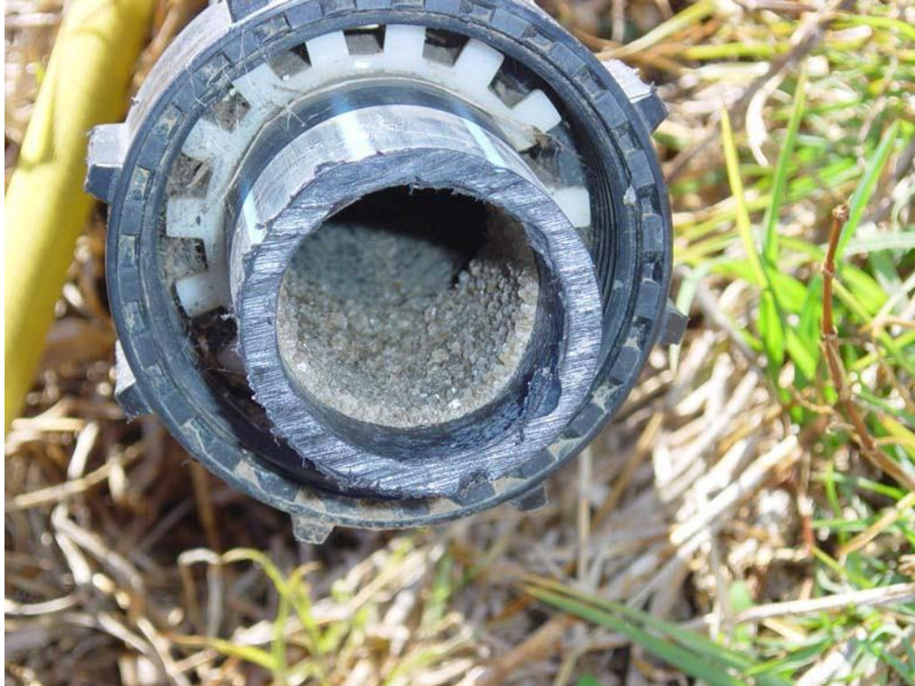
Crystalline 'Struvite' Build-up
